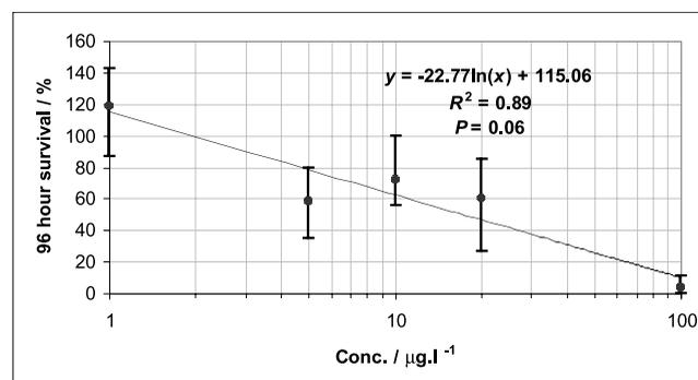
**Figure 2** | Dose response curve for chironomid larvae exposed to permethrin. The 96 h survival value represents the mean live:dead larvae ratio in the treatment as a percentage of the live:dead ratio in the control. Error bars represent range of triplicate experiments.
