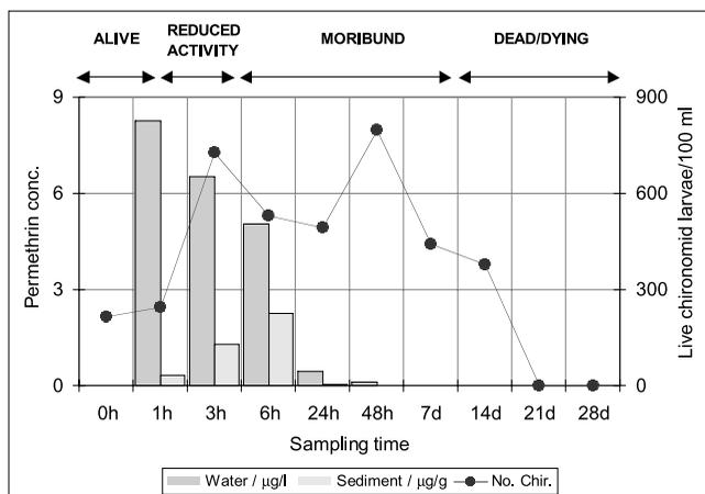
**Figure 3** | Numbers and status of live chironomid larvae in the schmutzdecke and corresponding mean concentrations ( $N=5$ ) of permethrin in the overlying water and the schmutzdecke.
