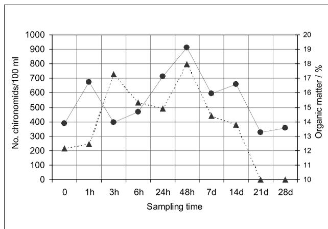
**Figure 4** | Organic matter content of the schmutzdecke and number of observed chironomid larvae. ● = mean no. chironomid larvae (N=5), ▲ = mean organic matter content (N=5).
