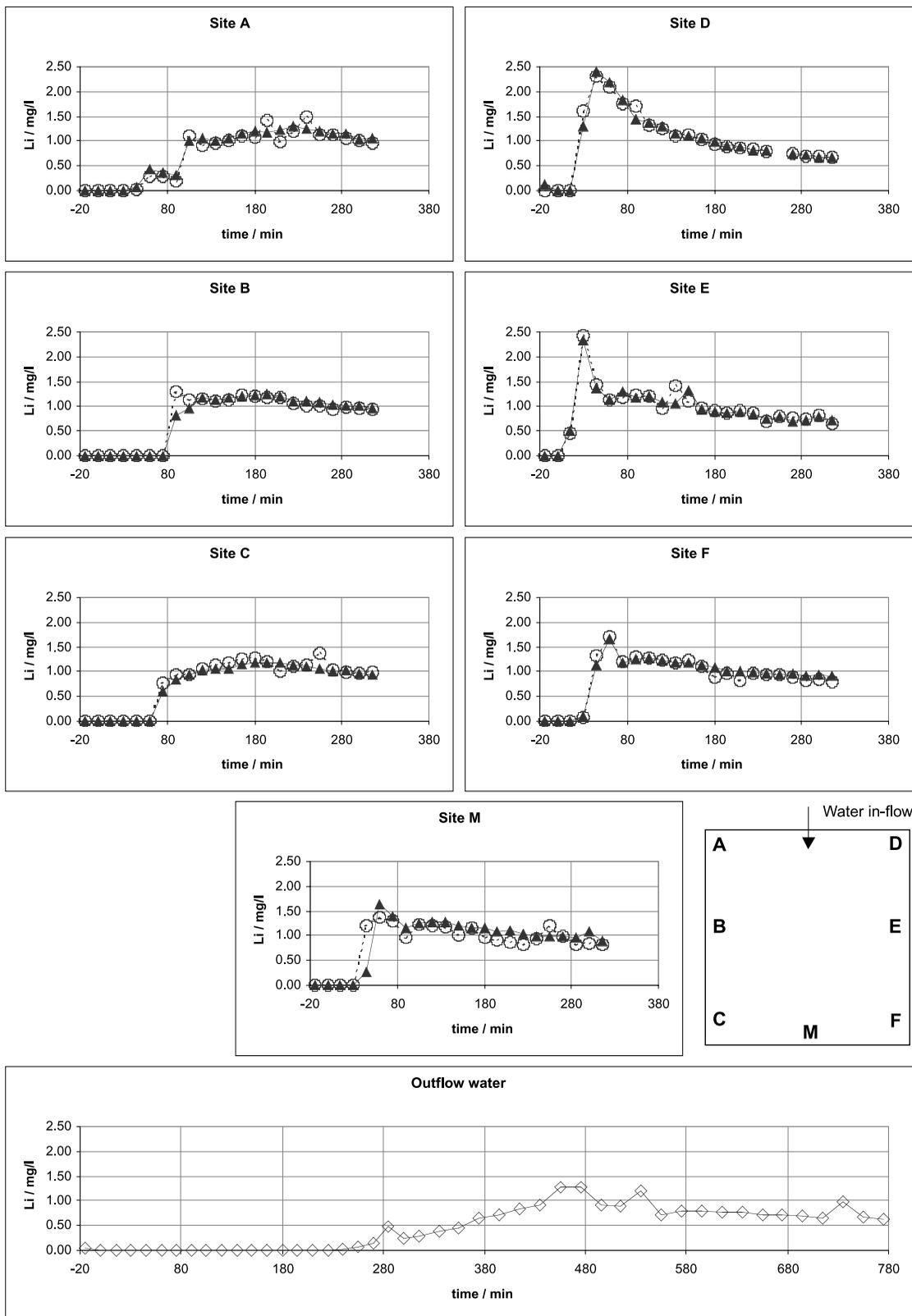
Figure 1 | Lithium concentrations and location of sampling positions in the slow sand filter bed. ▲=surface water, ○=bottom water, ◇=outflow water.
