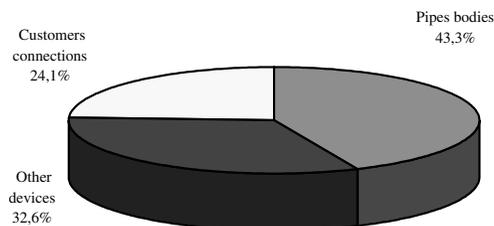
Figure 6 | Allocation of leaks to the system devices.
