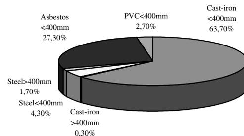
Figure 8 | Breaks allocation according to pipe material.
