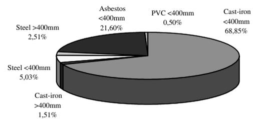
Figure 7 | Leaks allocation according to pipe material.
