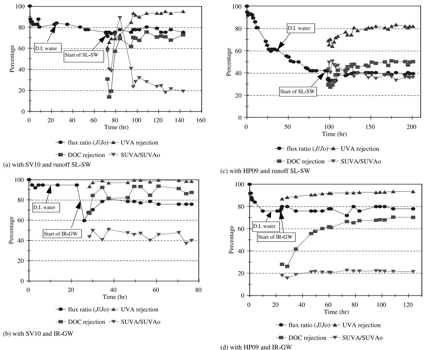
**Figure 7** | Flux-decline and NOM rejection of cross-flow membrane test.
