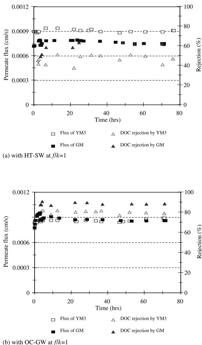
**Figure 4** | Hydrophobic interactions: YM3 vs. GM.
