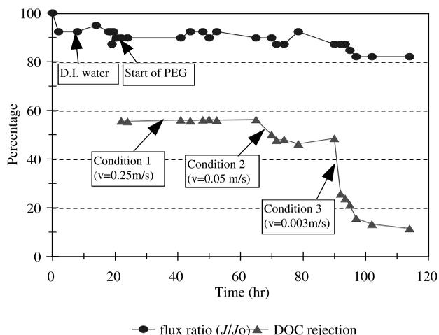
**Figure 8** | Flux decline and NOM rejection of cross-flow test with SV10 and PEG200.
