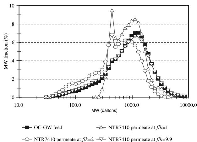
(d) by NTR7410 membrane with OC-GW at  $f/k=1.0$ ,  $2.0$ , and  $9.9$ **Figure 5** | MW distributions of permeates.
