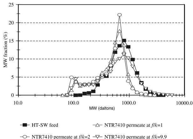
(b) by NTR7410 membrane with HT-SW at  $f/k=1.0$ ,  $2.0$ , and  $9.9$
