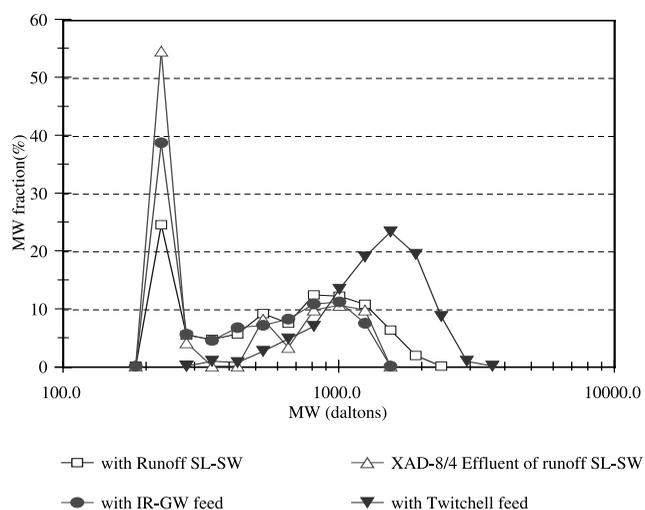
**Figure 6** | MW distributions comparison of permeates by GM membrane with different NOM sources.
