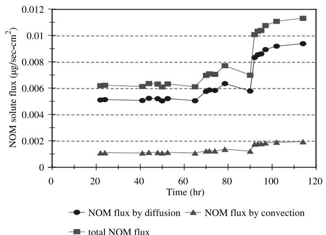
**Figure 9** | NOM transport of cross-flow test with SV10 and PEG200.
