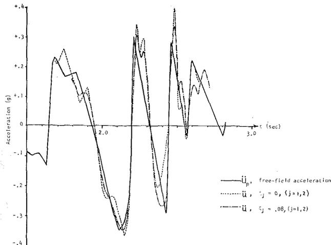
Fig. 2 Comparison of response for the two-mode PCRV with medium shear wave velocity at 4200 fps
