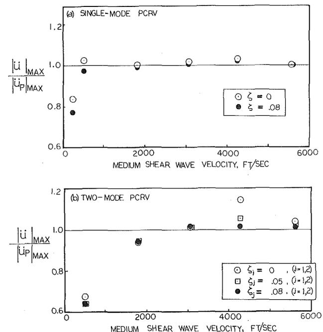
Fig. 1 Amplification factors of PCRv subjected to El Centro type earthquake
