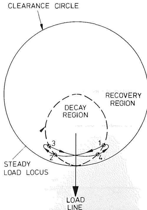
Fig. D3 Large decay region in circular bearings
