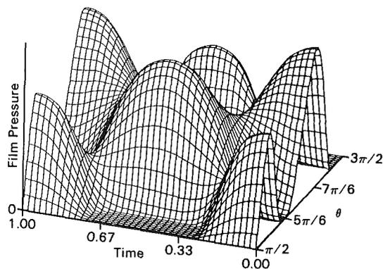
Fig. D5 Film pressure distribution around the bearing versus time for the optimum elliptical bearing
