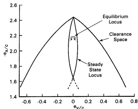
Fig. D4 Steady state and equilibrium loci for the optimum elliptical bearing
