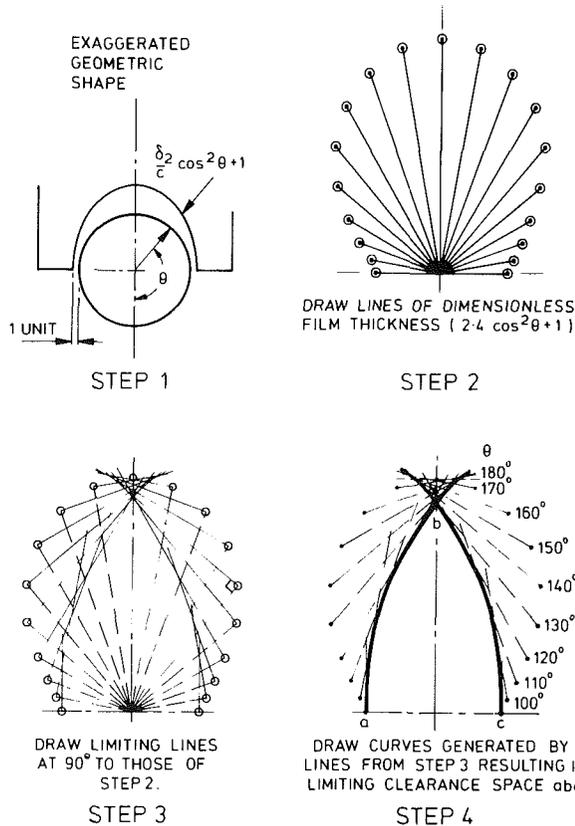
Fig. D1 Construction of limiting clearance shape for a noncircular bearing  $\delta_1/c = 0$ ;  $\delta_2/c = 2.4$
