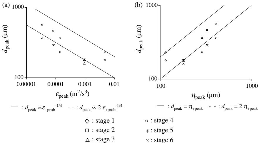
**Figure 6** Most probable floc size versus  $\varepsilon_{\text{peak}}$  (a) and  $\eta_{\text{peak}}$  (b)
