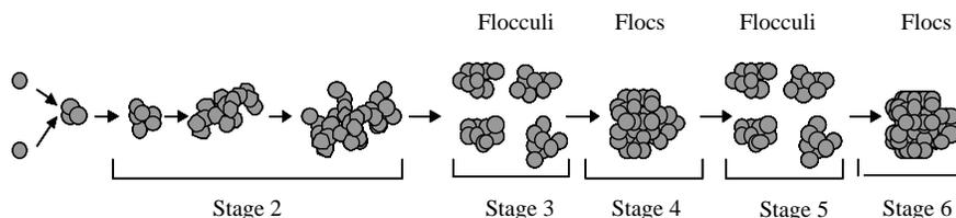
**Figure 8** Schematic of the evolution of floc structure during cycled flocculation
