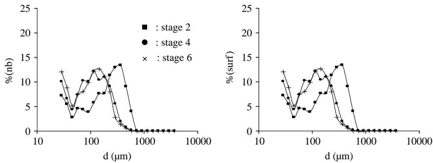
**Figure 3** Floc size distributions at the end of stages 2, 4 and 6 ( $\Omega_{\text{slow}} = 22 \text{ rpm}$ )
