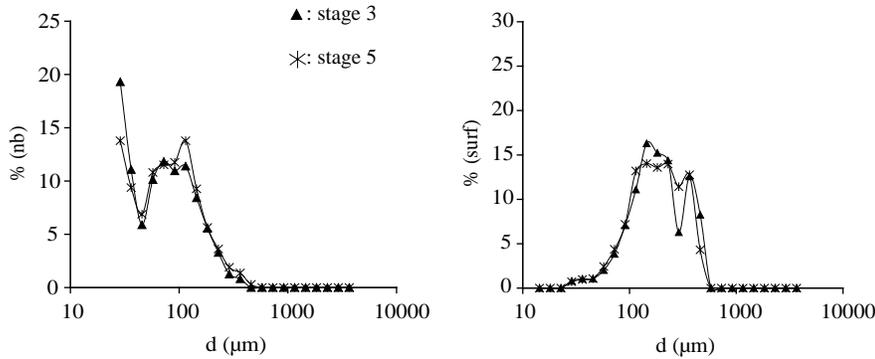
**Figure 5** Floc size distributions at the end of stages 3 and 5 ( $\Omega_{\text{slow}} = 22$  rpm)
