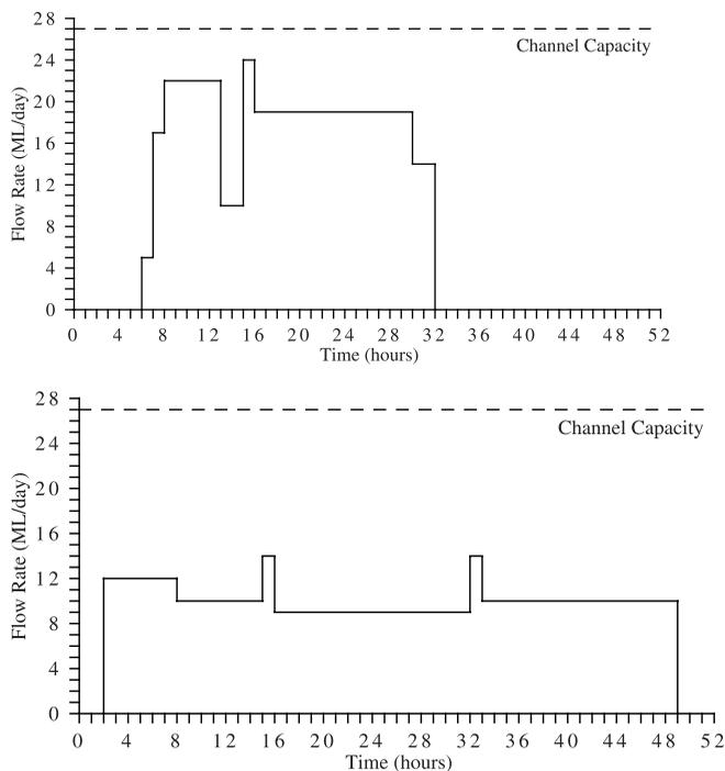
**Figure 10** | Case study flow rate time-series, for schedules: (a) requested by the irrigators; and (b) determined optimal by both exhaustive search and the GA. (a) string=[0,0,0,0,0],  $\Phi = -6.95$ , (b) string=[2,-5,0,17,0],  $\Phi = +52.7$ .
