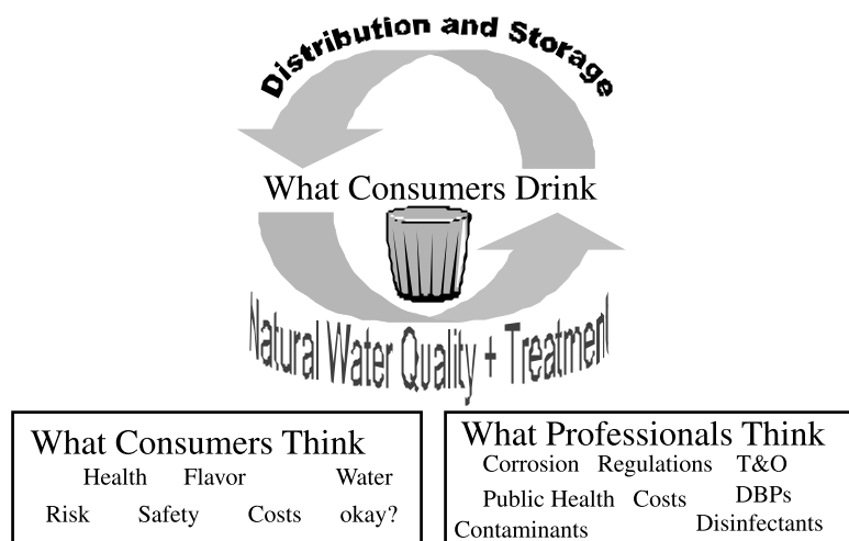
Figure 1 | Consumers use their senses and personal opinions to assess drinking water, the quality of which is determined by the raw water source, the treatment, and distribution according to regulated standards.
