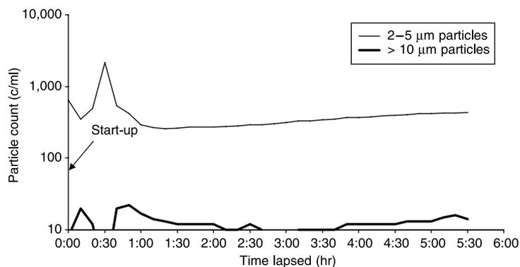
**Figure 2** | Spike in particle counts attributed to filter ripening following plant start-up at WTP 'A'.
