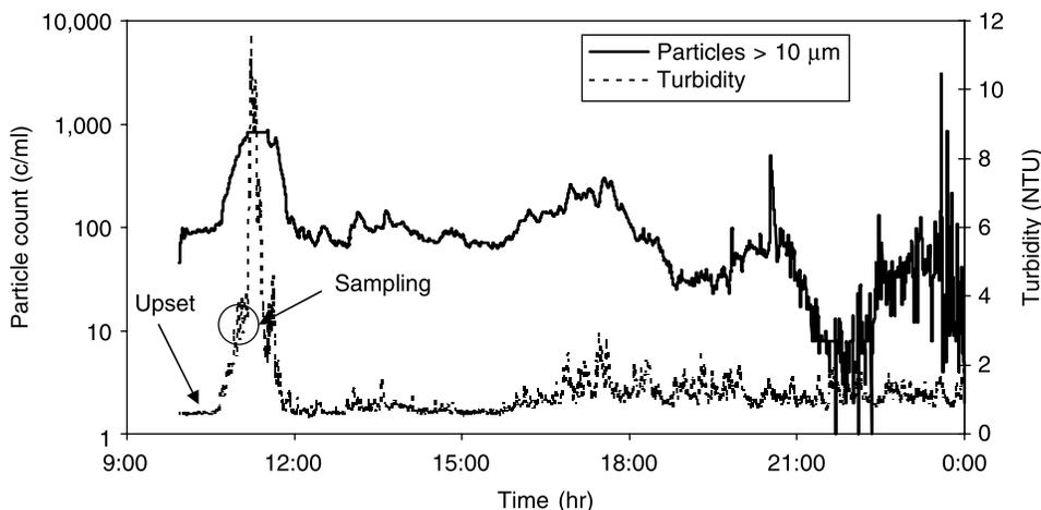
**Figure 8** | On-line monitoring data for particle counts  $>10 \mu\text{m}$  and turbidity after simulated upset in Actiflo® unit at WTP 'B'.
