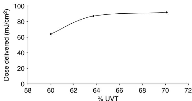
**Figure 6** | Dose delivered by pilot UV reactor for a range of %UVT observed at WTP 'A' based on MS2 biosimetry results.
