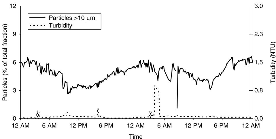
**Figure 4** | Typical % fraction of particles > 10 µm passing through pilot reactor at WTP 'A' over a sample 48 h duration.
