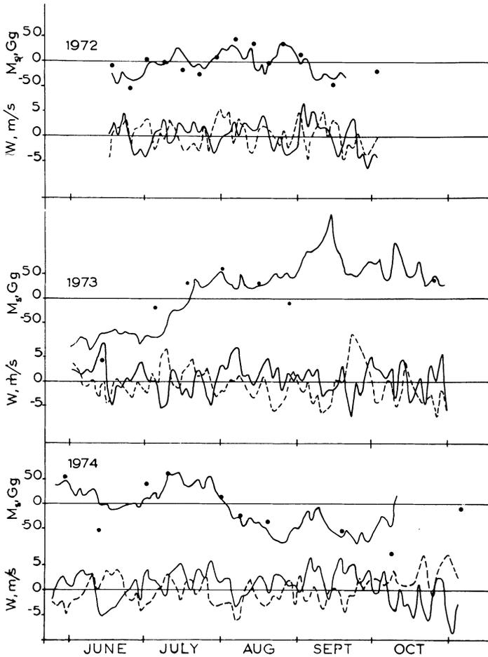
Fig. 6. The computed (heavy line) and measured (points) deviation of the salt content  $M_S$  from the mean value. The wind velocity  $W$  in the direction of Pohjanpitäjänlahti (positive to NE, heavy line) and perpendicular to this direction (positive to NW, broken line) is also presented.
