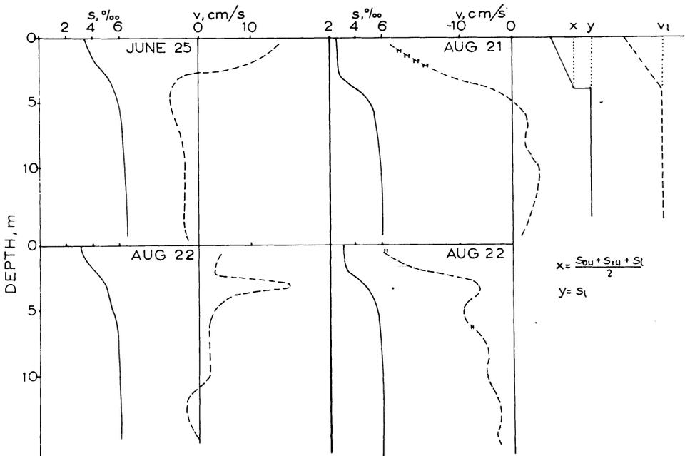
Fig. 4. Examples of distributions of salinity and velocity at point TK (1973). The diagram on the right represents the assumed velocity and salinity profiles. Positive velocity means inflow.
