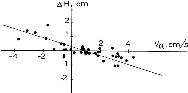
Fig. 5. The velocity  $V_{0\ell}$  plotted against the water level difference  $\Delta H$  at measuring points HT and HS. Each point marks the mean value of two days.
