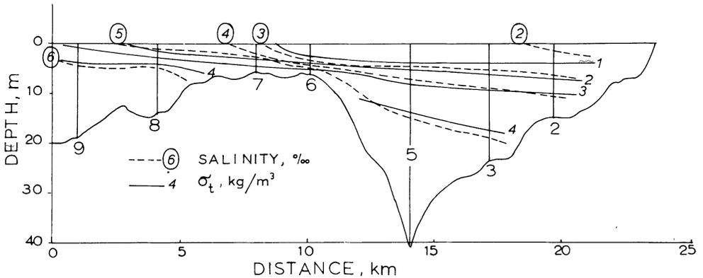
Fig. 2. The longitudinal section of Pohjanpitäjänlahti and Kaupunginselkä. Lines of equal salinity and density ( $\sigma_t$ ) correspond to mean conditions between May 22 and October 10 1973. The sounding points are numbered as in Fig. 1. Published by the permission of the Board of Navigation.
