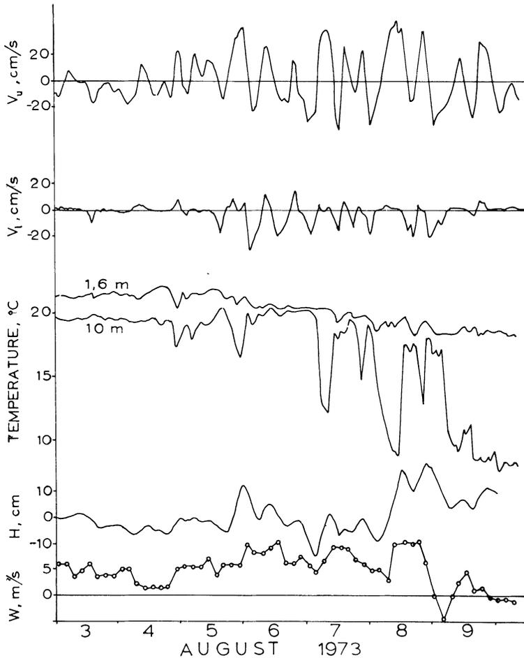
Fig. 3. An example of the hourly mean values of flow velocities at point CV, and water level  $H$  at HZ. The component of the wind velocity  $W$  along the direction of Pohjanpitäjänlahti measured at Russarö island is also given. The positive direction of the wind velocity is to the NE.
