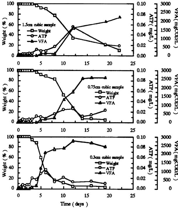
Figure 2 Changes of weight, ATP and VFA and concentrations in case of carbohydrate solid samples
