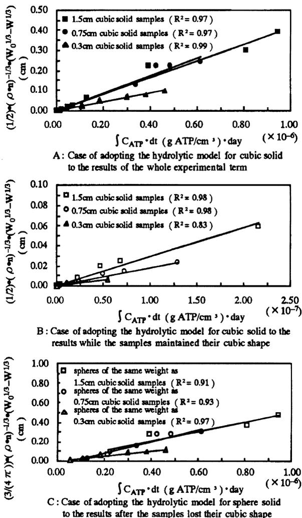
**Figure 7** Analysis of the degradation of carbohydrate solid samples by the hydrolytic model on surface area basis
