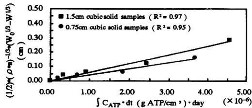
A: Case of adopting the hydrolytic model for cubic solid to the results of the whole experimental term
