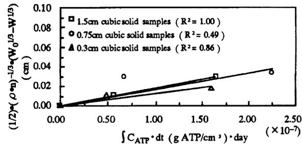
B: Case of adopting the hydrolytic model for cubic solid to the results while the samples maintained their cubic shape
