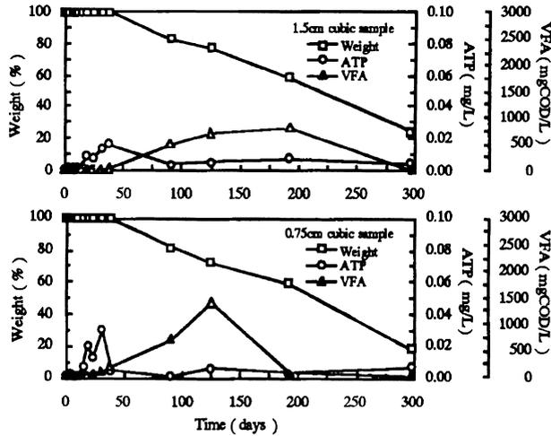
Figure 4 Changes of weight, ATP and VFA concentrations in case of lipid solid samples
