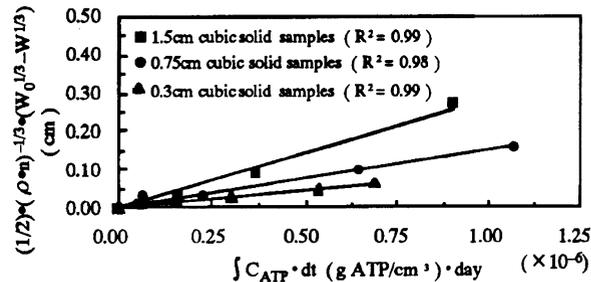
A: Case of adopting the hydrolytic model for cubic solid to the results of the whole experimental term
