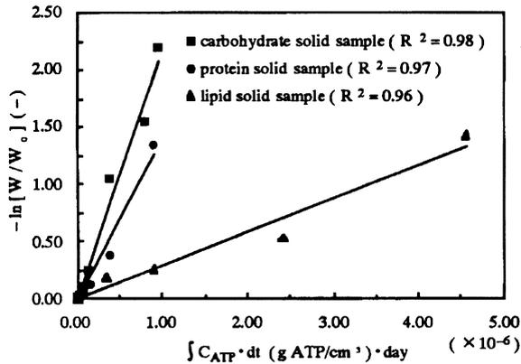
Figure 5 Analyses of the degradation of organic solid samples by the hydrolysis model based on solid weight
