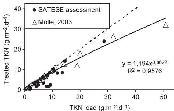
**Figure 8** Treated TKN on 2<sup>nd</sup> stage ( $0.05 < \text{HL} < 2.2 \text{ m.d}^{-1}$ )
