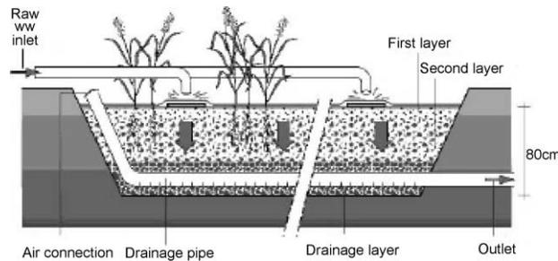
**Figure 1** A typical 1<sup>st</sup> stage RBF
