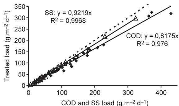
**Figure 4** Treated COD and SS for COD concentrations between 520–1400 mg.L<sup>-1</sup>; 0.15 < HL < 0.6 m.d<sup>-1</sup>
