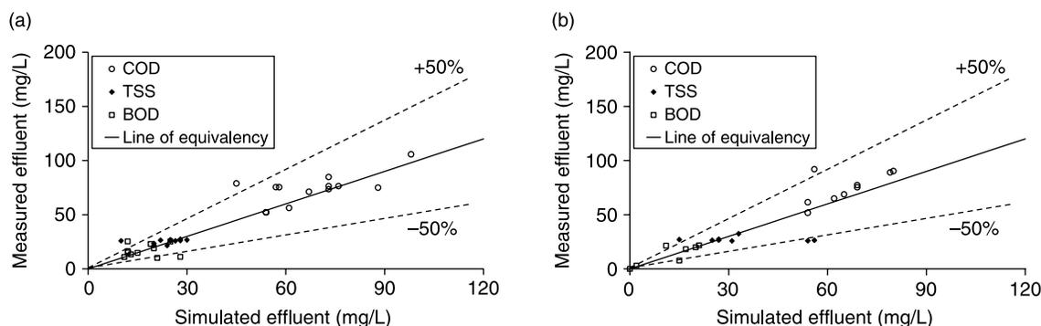
**Figure 4** | Results of model calibration (a) and validation (b) in terms of COD, TSS, BOD concentrations at the WWTP outflow.
