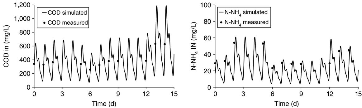
**Figure 5** | Measured and simulated input series for the 15-days simulation of the HMBBR system in term of COD and N-NH<sub>4</sub>.
