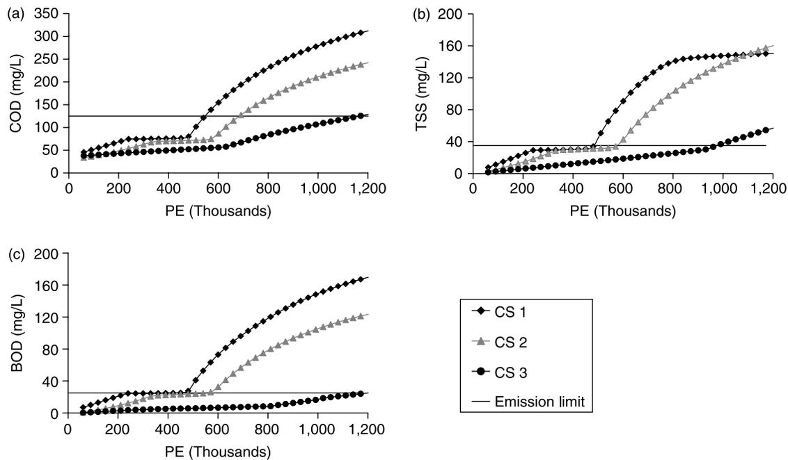
Figure 7 | CS comparisons, a, b, and c, respectively, for COD, TSS and BOD.
