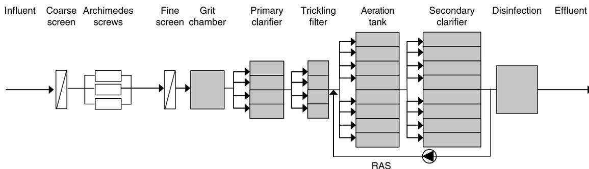
Figure 1 | Layout of Acqua dei Corsari wastewater processing.
