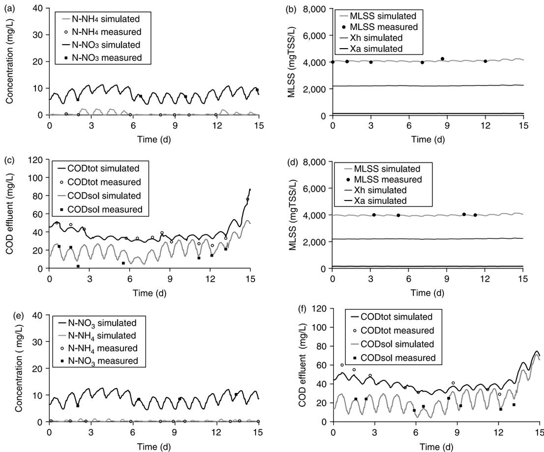
**Figure 6** | Model results for the HMBBR pilot plant with different filling rates of 35% (a, b, and c) and 66% (d, e and f).
