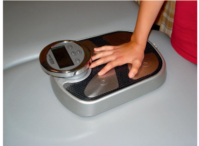
Figure 4. Compression of the padding of a table simulates the soft tissue of the body. The scale measures the force needed to compress this during mobilization simulation.
