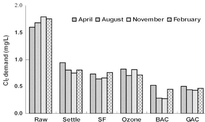
Figure 4 Chlorine demand on each process
