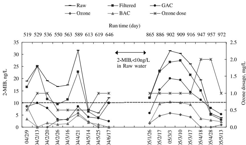
**Figure 3** 2-MIB concentration in each process during low temperature period
