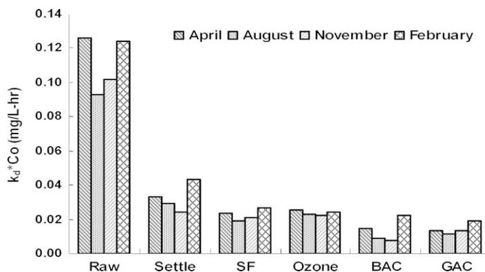
Figure 5 Chlorine decay rates on each process
