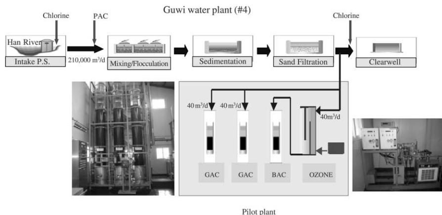
Figure 1 Schematic of pilot plant
