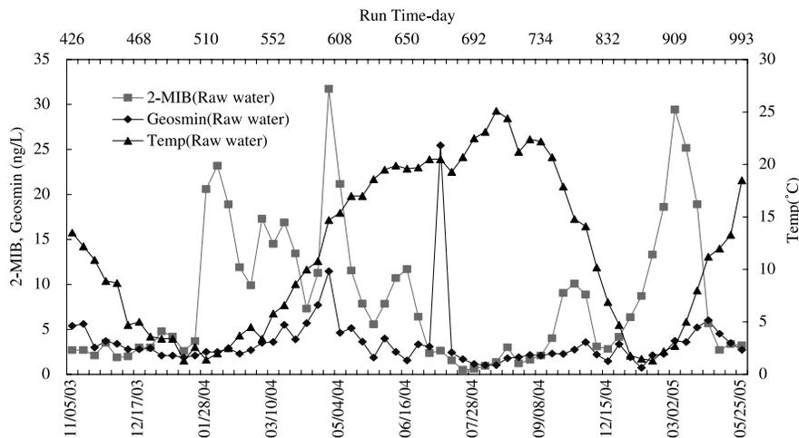
**Figure 2** 2-MIB and geosmin concentrations in the raw water with water temperature
