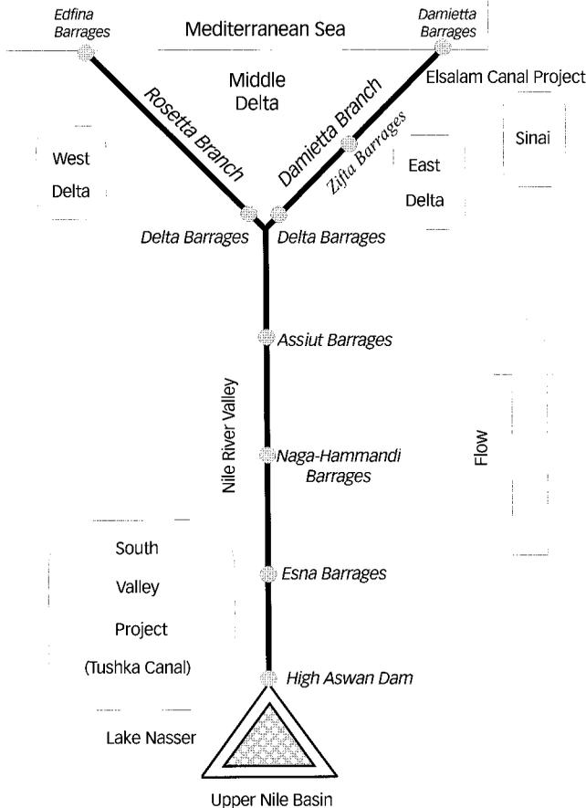
Figure 4 | Schematic diagram of the water system in Egypt.
