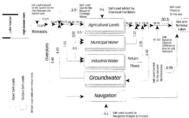
Figure 6 | The salt balance for the system.
