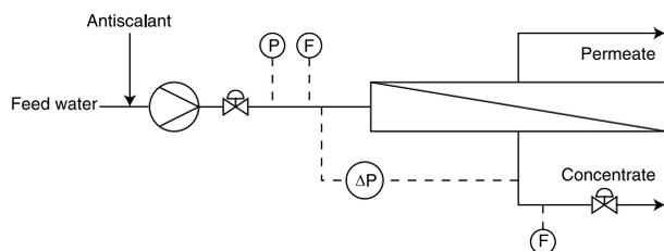
**Figure 2** | Simplified flowsheet of one of the pilots used for the experiments with 4" modules. Antiscalant was dosed to the feed water and a pump was used to pressurize the feed water. Feed pressure (P), flow (F) and pressure drop along the module ( $\Delta P$ ) were measured. The desired recovery of the system of 20% was set with control valves in the concentrate and feed lines.
