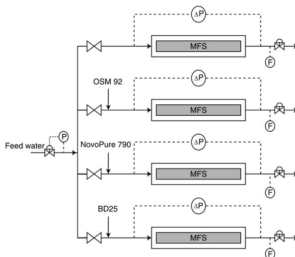
**Figure 1** | Flowsheet of the four parallel MFS flowcells. All cells can be operated independently, but are fed by the same feed water at the same pressure. Flows (F) and pressure differences ( $\Delta\text{P}$ ) are measured and controlled for each cell.
