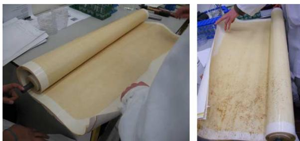
**Figure 7** | Photographs from the membrane autopsies performed for the two elements. The left photo shows the element operated with BD25, the right photo shows the element operated with NovoPure 790. In the right photo, the feed water flowed from bottom to the top.
