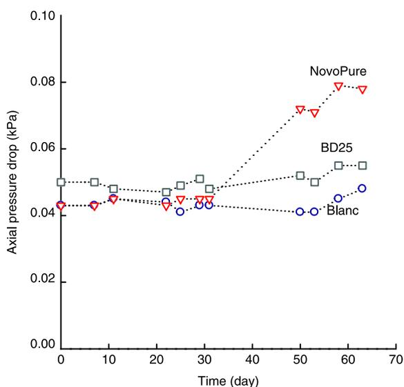
**Figure 4** | Development of the axial pressure drop in three MFS cells operated for 63 days with two different antiscalants and a blank run with no added chemicals. The cell operated with NovoPure 790 (triangles) showed a strong increase in the axial pressure drop after 35–45 days of operation. The module operated with BD25 only showed a minor increase in axial pressure drop towards the end of the experiment, similar to the increase observed for the blank.
