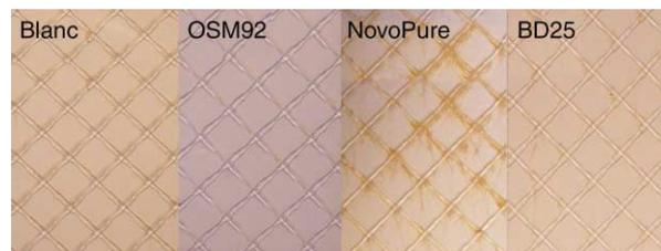
**Figure 3** | Images of the membrane and spacer from the MFS cells after 63 days of operation while dosing different antiscalants. Differences in colours of the membranes were due to different lighting conditions. The blank and the membrane in the cell operated with BD25 showed minor mass accumulation. The MFS cell operated with NovoPure 790 showed severe mass accumulation. The cell operated with the standard antiscalant (OSM 92) showed negligible mass accumulation.
