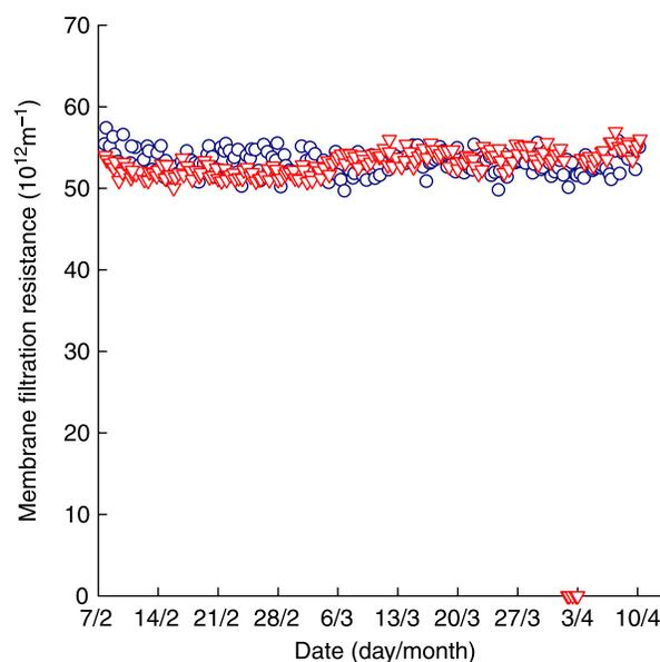
**Figure 6** | Filtration resistance for the two 4" pilot modules over the testing period of 63 days. No significant changes in membrane resistance were observed for the module operated with NovoPure 790 antiscalant (triangles) nor for the module operated with BD25 (circles).
