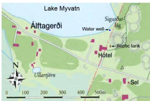
Figure 2 | Study site. Map of the study area (adapted from Jonsson (2006)). The water well and the septic tank are marked. The hotel and six dwelling houses are served by the well, four at Álfagerði and two close to the hotel.
