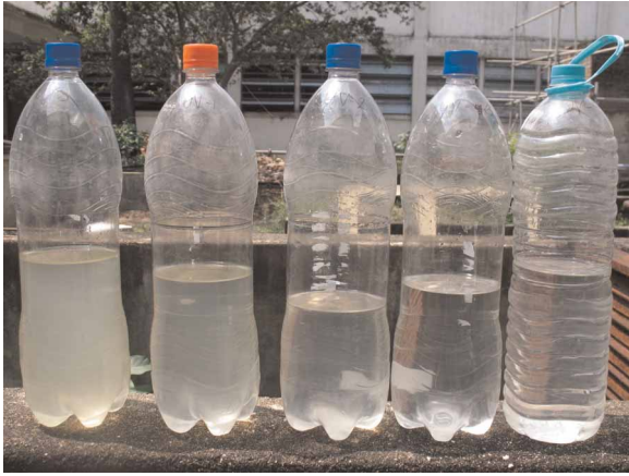
Figure 3 | Bottles ready to be subjected to SODIS. L to R: SODIS-only control, sari-filtration-only control (Jar 1), sub-optimal moringa dose (Jar 2), optimal moringa dose (Jar 3) and supra-optimal dose (Jar 4).
