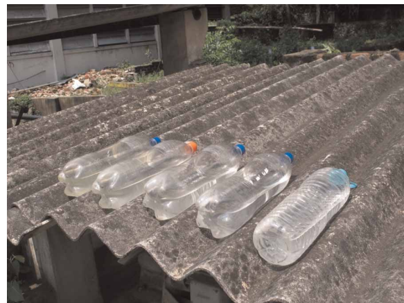
Figure 2 | Bottles placed on inclined roof surface for SODIS stage.
