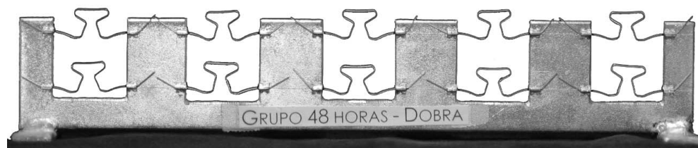
Figure 4. Structure simulating a clinical situation used for adaptation of springs in different times. From Caldas et al., Effects of stress relaxation in beta-titanium orthodontic loops. Am J Orthod Dentofacial Orthop. 2011;140:e85–e92. Courtesy of Elsevier Inc.
