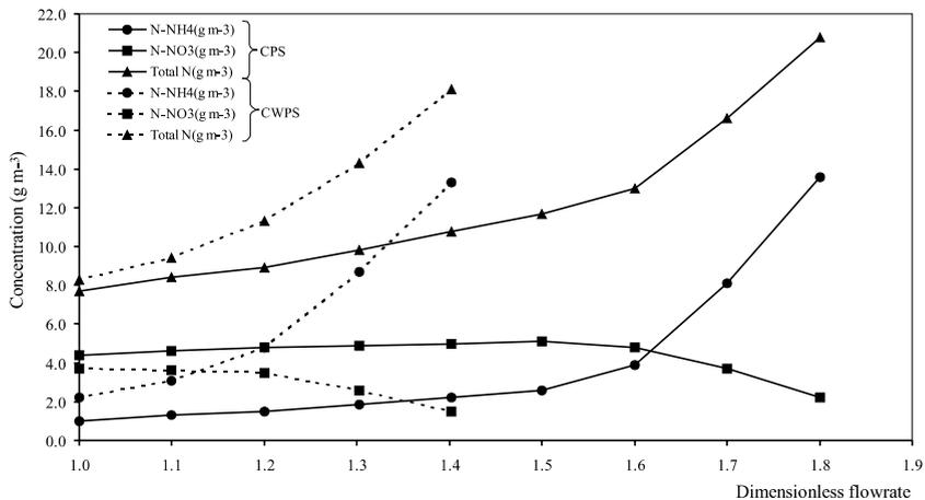
Figure 2 Nitrogen compounds concentration in the effluent versus dimensionless flowrate
