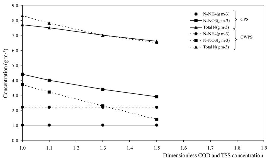
**Figure 4** Nitrogen compounds concentration in the effluent versus dimensionless COD and TSS
