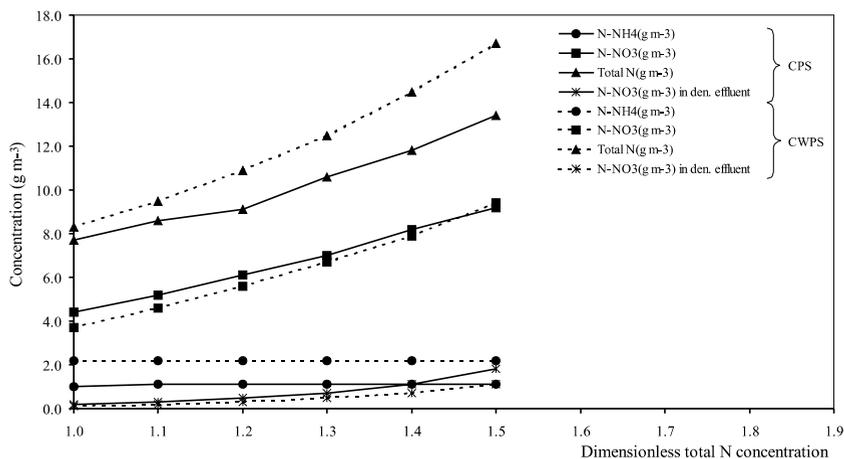
**Figure 3** Nitrogen compounds concentration in the effluent versus dimensionless total N
