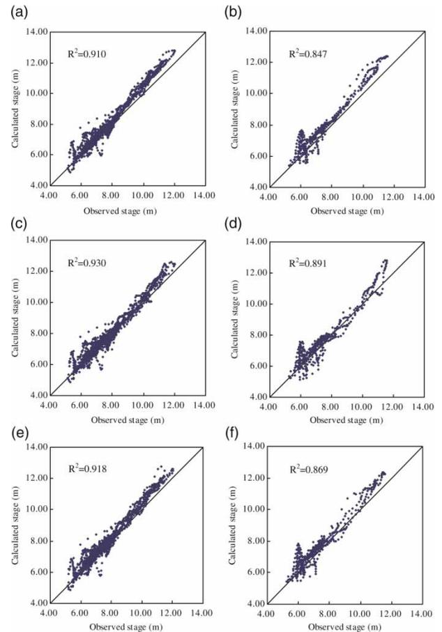
Figure 6 | Comparison of observed and calculated stages with calibrated  $\alpha$  at Zhaixi in the Qiantang River: (a) calibration results with SVN model; (b) validation results with SVN model; (c) calibration results with SVN-1 model; (d) validation results with SVN-1 model; (e) calibration results with SVN-2 model; and (f) validation results with SVN-2 model.
