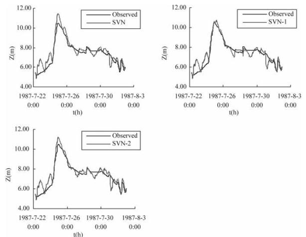
**Figure 3** | Stage hydrograph of flood 870722 at Zhaixi in the Qiantang River.
