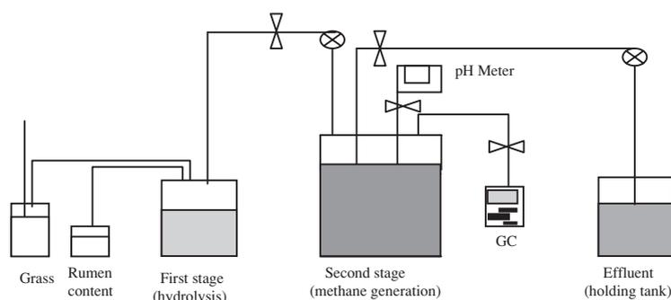
**Figure 1** Schematic representation of the experimental unit
