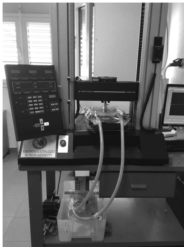
Figure 2. Hydraulic circuit to keep the temperature constant.
