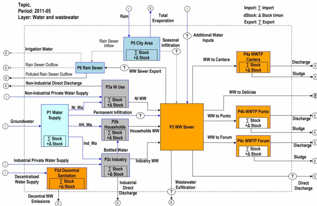
Figure 1 | Model setup for the MFA of year 2011 at the case study city. Abbreviations: E—export, HH—household, I—import, NI—non-industrial, Wa—drinking water, WW—wastewater, WWTP—wastewater treatment plant. A '?' symbol is shown at flows which have not been assessed before at the location.
