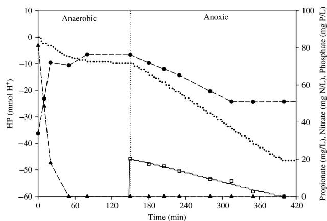
**Figure 1** | Typical SBR anaerobic-anoxic cycle with nitrate as electron acceptor monitored with titrimetric measurements (dotted line). Off-line measurements: propionic acid ( $\blacktriangle$ ), nitrate ( $\square$ ) and phosphate ( $\bullet$ ). The estimation of nitrate concentration based on HP measurements is represented with a solid line.
