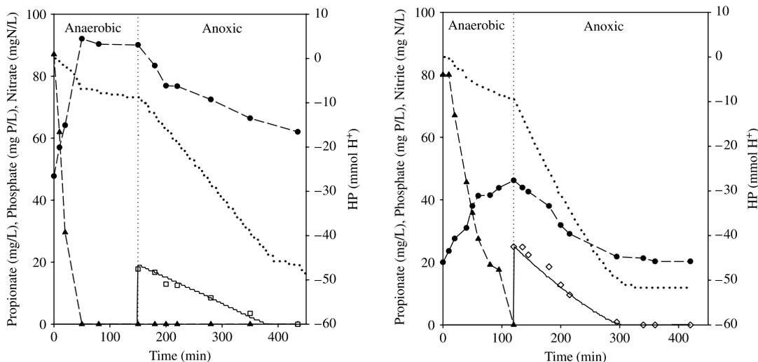
**Figure 3** | Typical SBR anaerobic–anoxic cycles monitored with titrimetric measurements (dotted line). Off-line measurements: propionic acid (▲), nitrate (□), nitrite (◇) and phosphate (●). The estimations of nitrate and nitrite concentration based on HP measurements are shown with a solid line.
