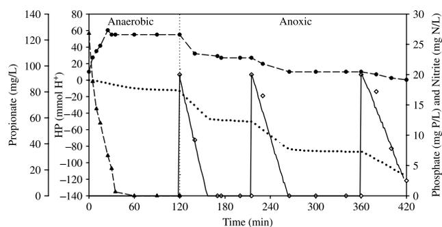
**Figure 2** | Typical SBR anaerobic-anoxic cycle with nitrite as electron acceptor monitored with titrimetric measurements (dotted line). Off-line measurements: propionic acid ( $\blacktriangle$ ), nitrite ( $\diamond$ ) and phosphate ( $\bullet$ ). The estimation of nitrite concentration based on HP measurements is represented with a solid line.
