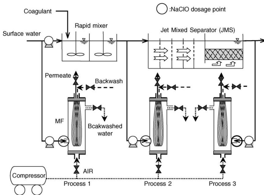
**Figure 2** Schematic diagram of the pilot-scale apparatus; process 1), 2), and 3)
