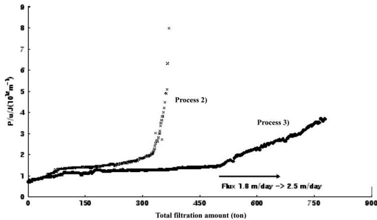
Figure 4 Variation of filtration resistance in process 2) and 3)
