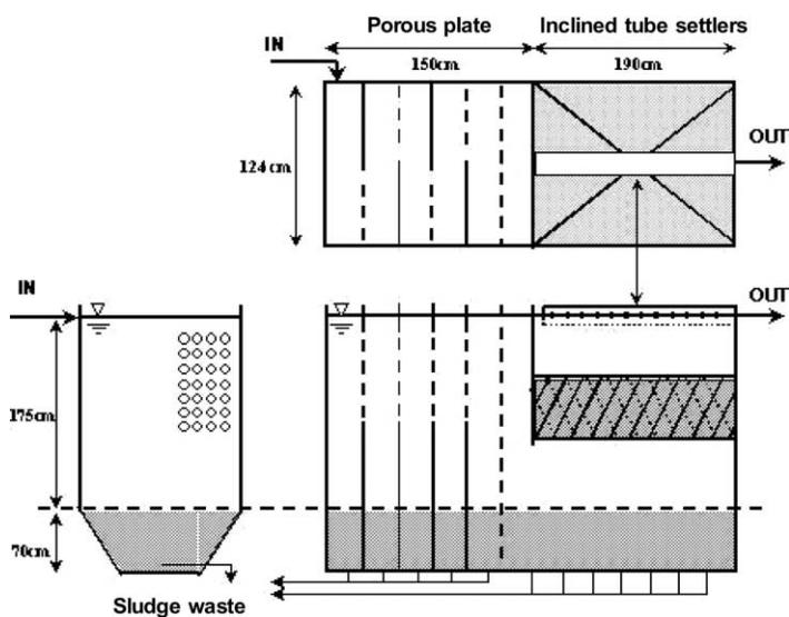
**Figure 1** Schematic diagram of the Jet Mixed Separator (JMS)
