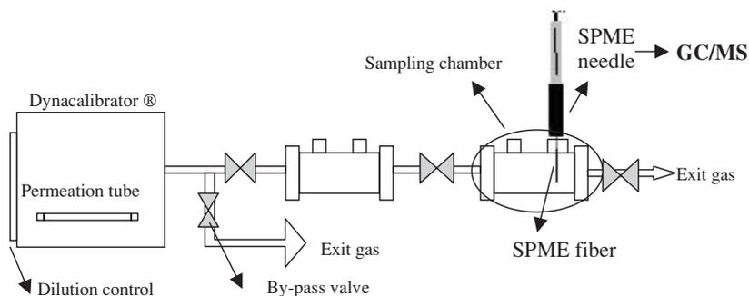
**Figure 1** Set-up used for SPME calibration for odor analysis
