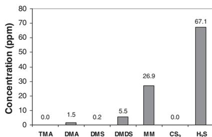
**Figure 5** Odor concentrations in a digested biosolids sample measured using the SPME–GC–MS method. Concentrations of TMA and CS<sub>2</sub> were below detection
