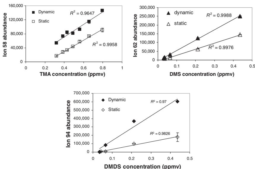
**Figure 2** Response under dynamic and static sampling modes for TMA, DMS, and DMDS
