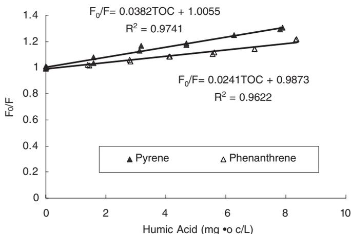
**Figure 2** The sorption coefficient of PAHs onto humic acid (3,000 Da filtrate)
