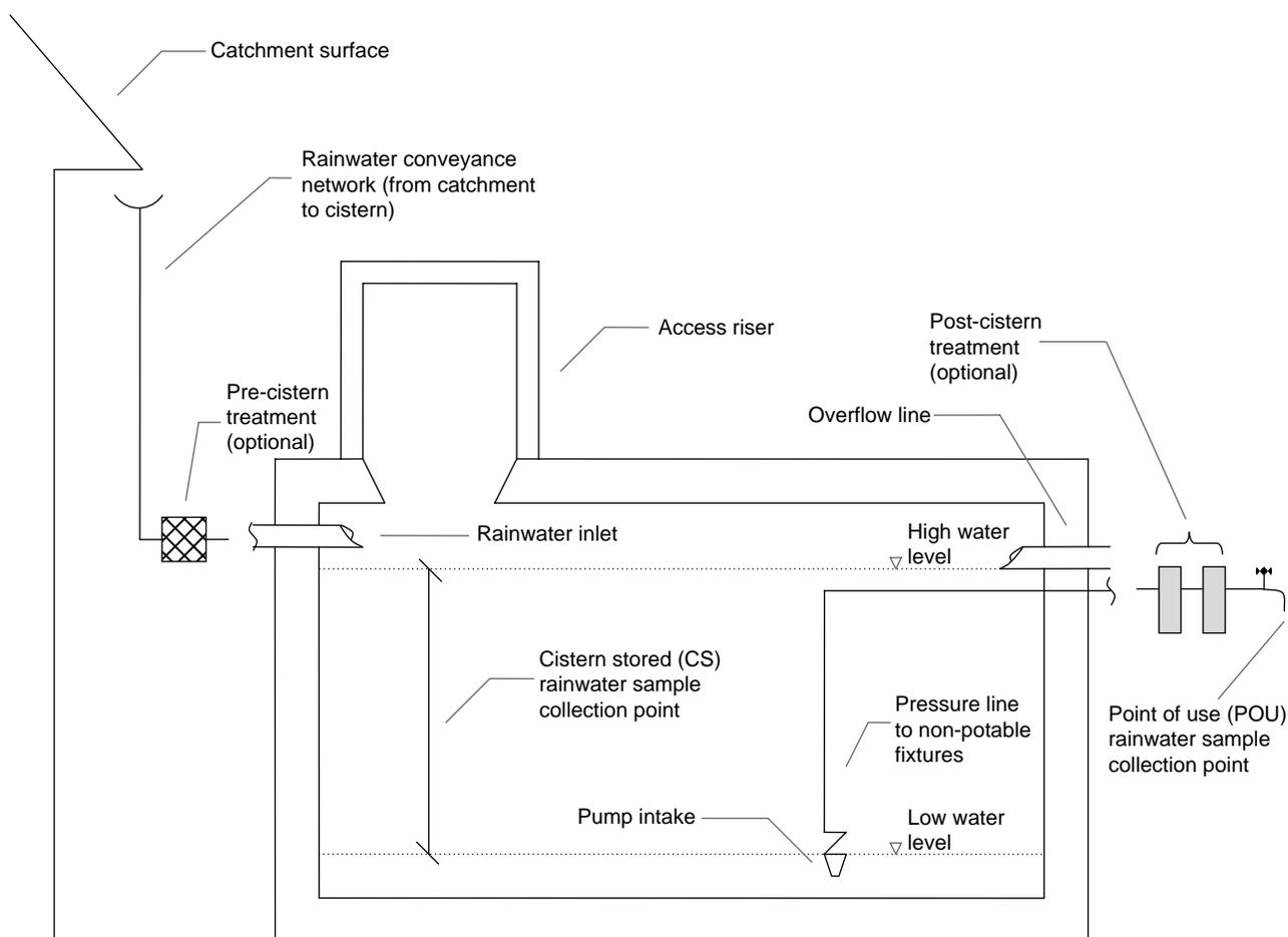
Figure 3 | Representative schematic of interior of rainwater cistern (section view).
