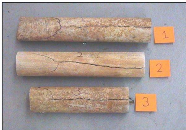
Figure 4 | Failed asbestos cement pipe sections.
