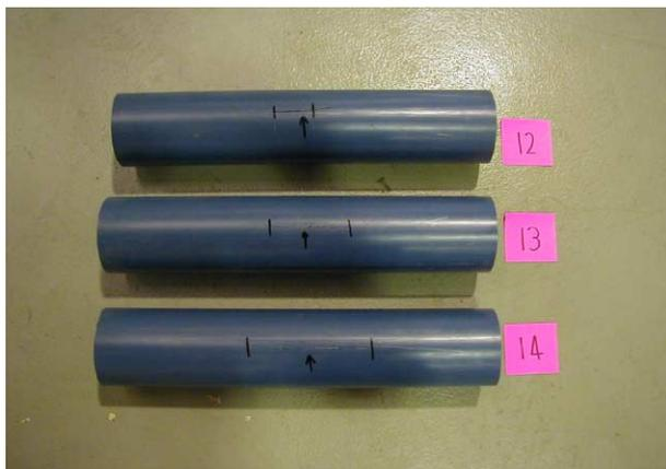
Figure 10 | Longitudinal cracks in uPVC.
