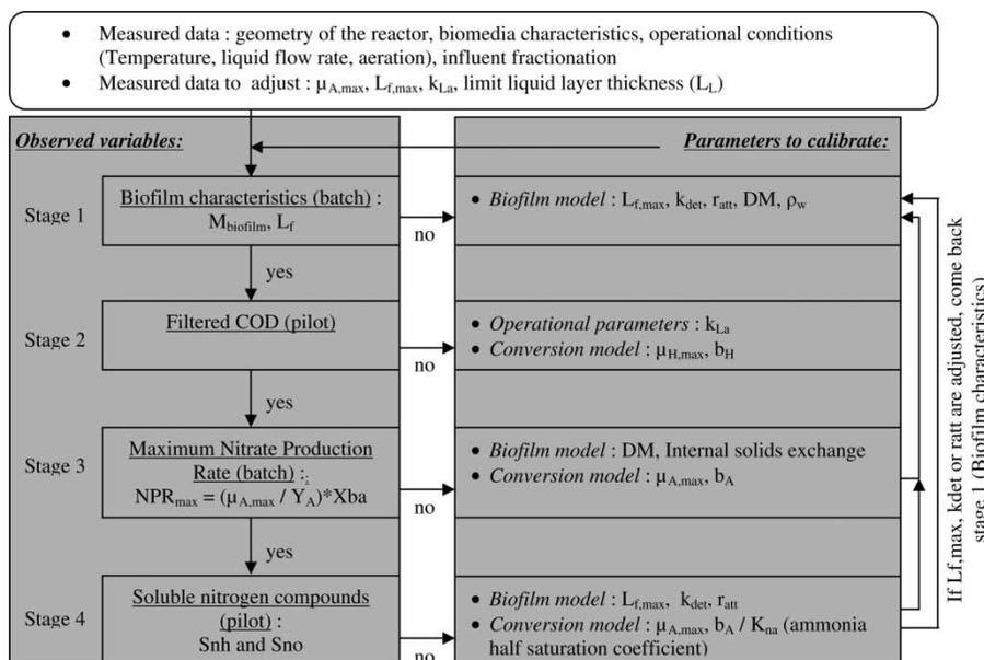
Figure 3 | Calibration procedure of MBBR 1D-model in reactor N.
