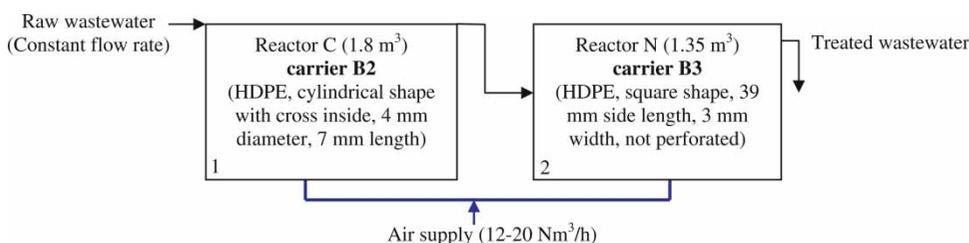
Figure 1 | Schematic representation of the pilot-scale plant.
