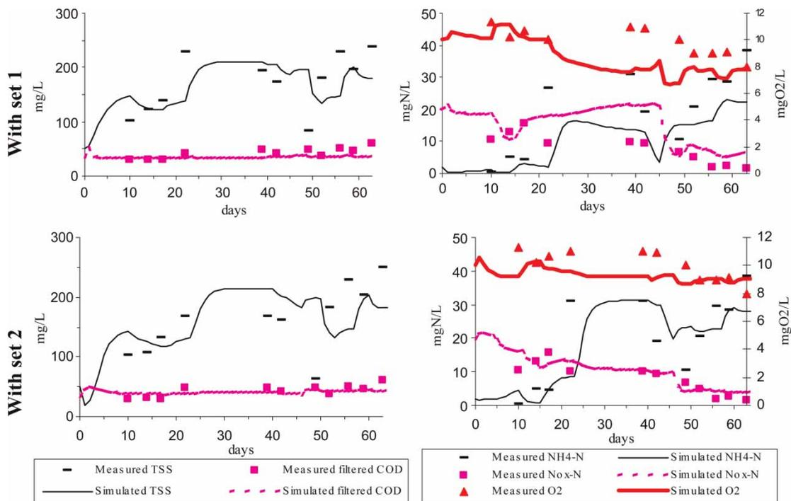
**Figure 4** | Measured and simulated reactor N effluent concentrations with set 1 and set 2.
