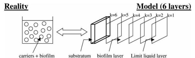
Figure 2 | Schematic representation of one-dimensional MBBR model (from Hydromantis 2006).
