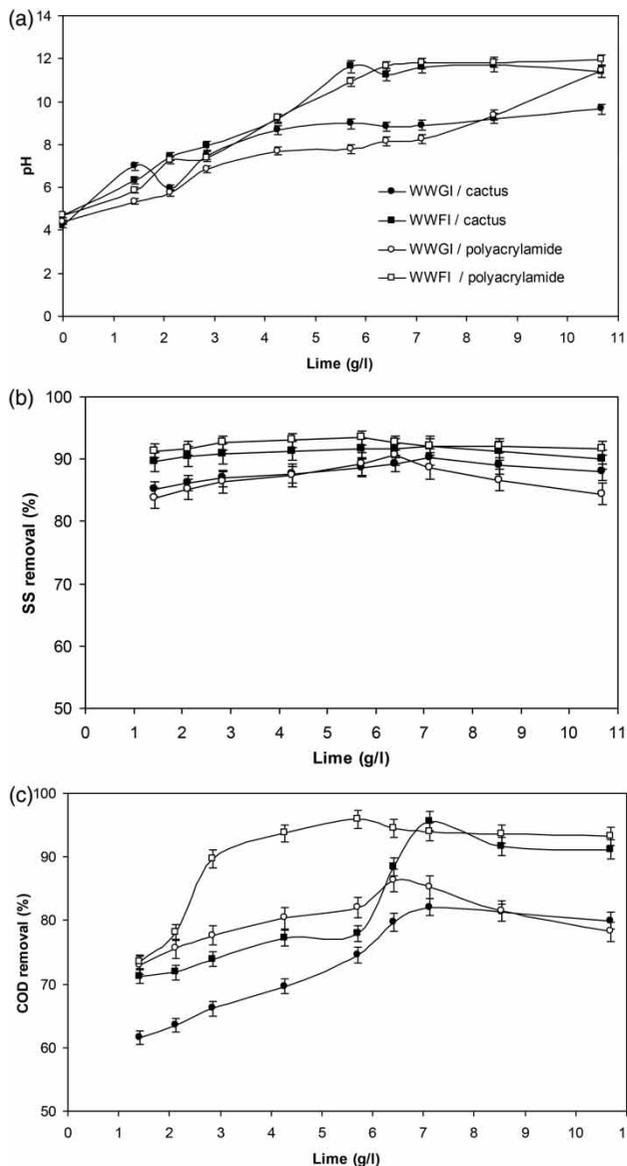
**Figure 2** | The effect of lime on coagulation–flocculation performance in the presence of optimum doses of CJ (0.056 and 0.616 g/L, respectively, for WWFI and WWGI) and PAM (0.028 and 0.076 g/L, respectively, for WWFI and WWGI) used as flocculant: (a) pH variations; (b) SS removal; (c) COD removal.
