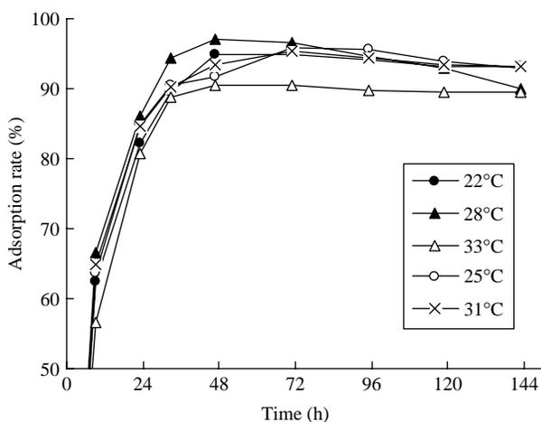
Figure 2 | Effect of temperature of  $Mn^{2+}$  on adsorption rate.
