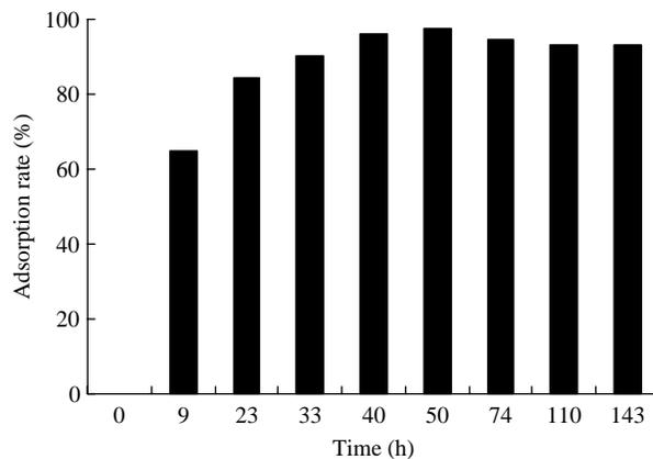
Figure 7 | The adsorption rate change curve of A5 at optimal conditions.
