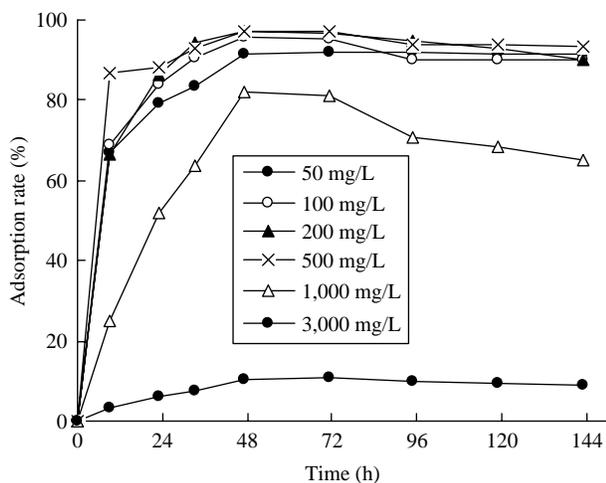
Figure 3 | Effect of the initial concentration of  $Mn^{2+}$  on adsorption rate.
