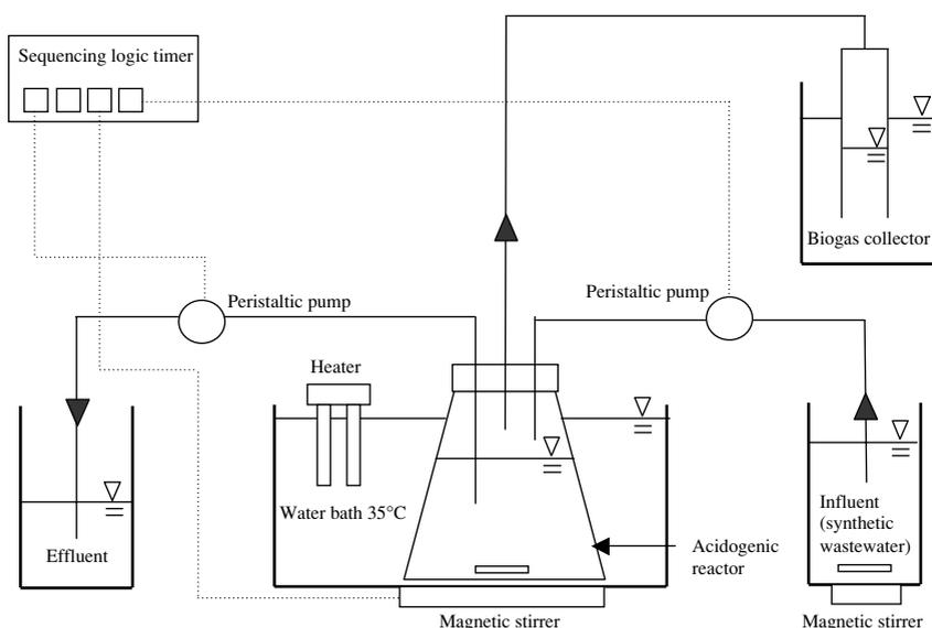
**Figure 1** Experimental setup of the acidogenic sequencing batch reactor
