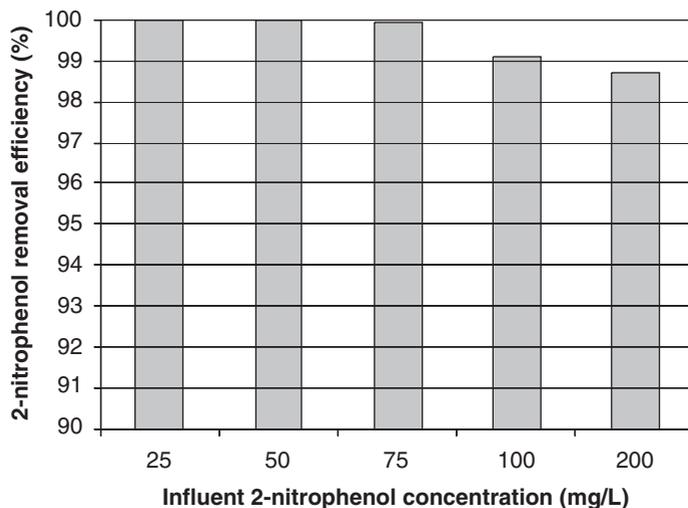
**Figure 2** Removal efficiency of 2-nitrophenol at different concentrations
