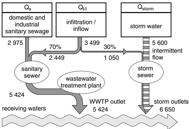
**Figure 3** Idealized separate sewer system with average flow rates in  $m^3/(ha_{imp} \cdot a)$  according to Table 1
