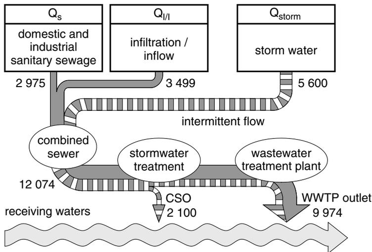
**Figure 2** Idealised combined sewer system with average flow rates in  $m^3/(ha_{imp} \cdot a)$  according to Table 1
