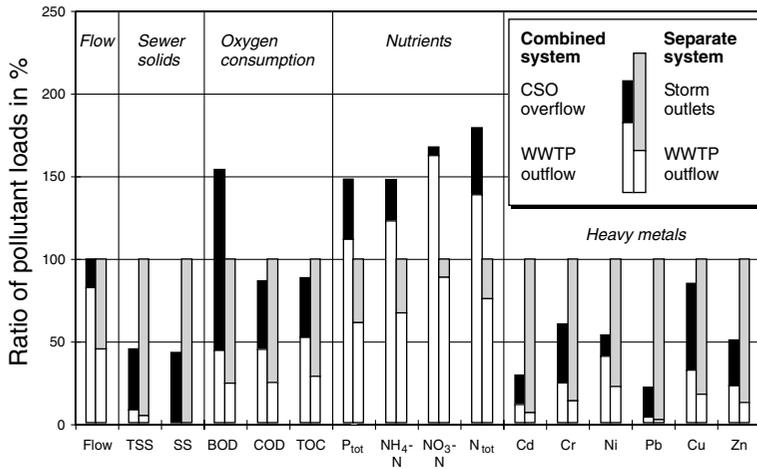
**Figure 6** Ratio of pollutant loads; all loads are standardized using the total load (storm outlets plus treatment plant outflow) from a separate system as 100%. The white columns indicate the share of the WWTP outflow load
