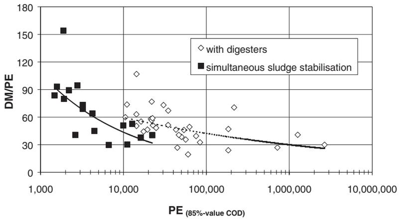
**Figure 4** Specific annual costs for biological treatment, sludge stabilisation and sludge disposal on plants with extra sludge digesters and simultaneous stabilisation plants
