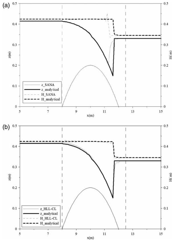
**Figure 8** | (a) Water level (lower curve) and total head (upper dashed curve) for the bump test case: SANA (grey line) and analytical solution (black line). (b) Water level (lower curve) and total head (upper dashed curve) for the bump test case: HLL-CL (grey line) and analytical solution (black line).
