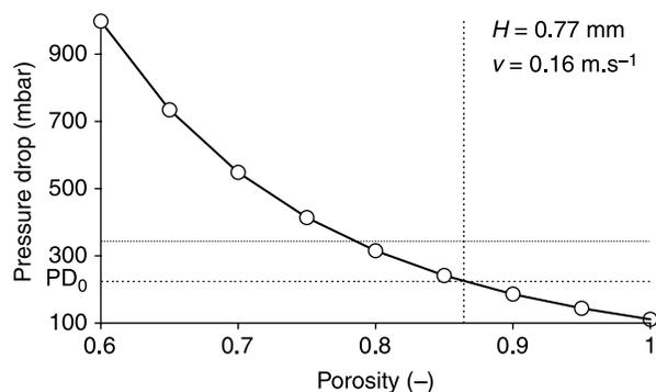
**Figure 1** | Feed channel pressure drop in relation to the increase of the porosity of the feed spacer of a 2540-type membrane element.  $H$  = feed channel height;  $v$  = feed flow velocity;  $PD_0$  = feed channel pressure drop for a clean membrane element.
