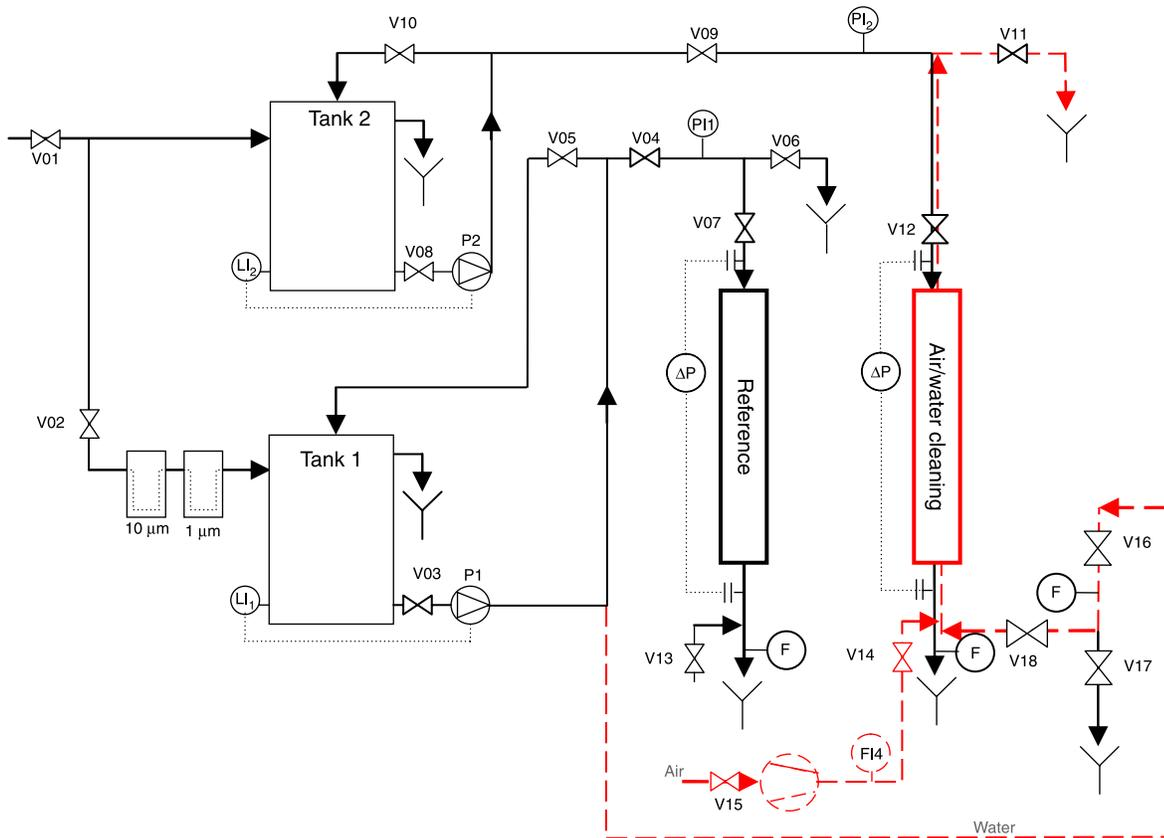
**Figure 2** | Schematic diagram of pilot setup for air/water cleaning.
