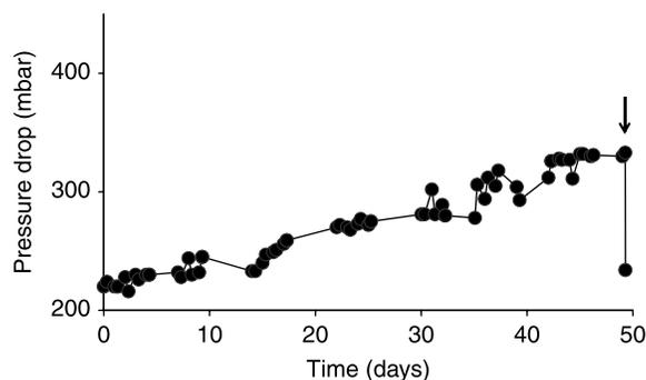
**Figure 5** | Pressure drop development along the membrane channel of the reference element (REF) without air/water cleaning. At day 50 a 5-minute air/water cleaning was carried out (indicated by the arrow).
