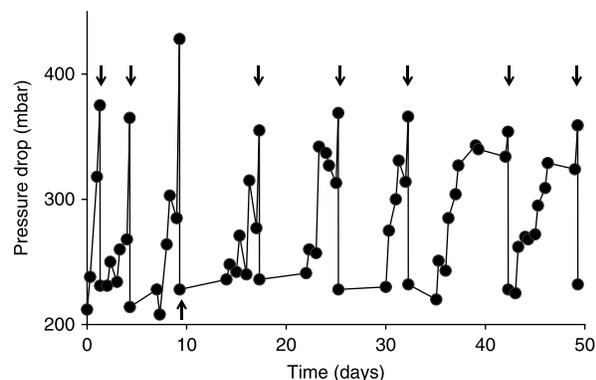
**Figure 6** | Pressure drop development along the membrane channel of air/water cleaned membrane element (AWC). A total of eight air/water cleanings, each lasting for 5 minutes, were carried out in the 50-day experiment (as indicated by the arrows).
