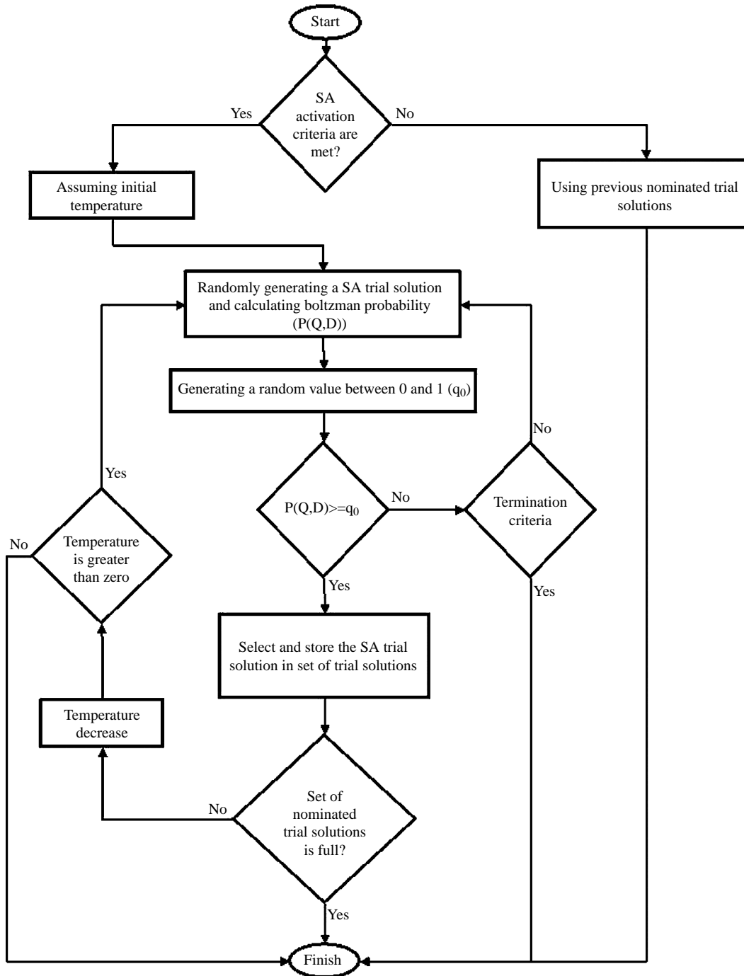
Figure 4 | SA process flowchart in the improved HBMO algorithm.
