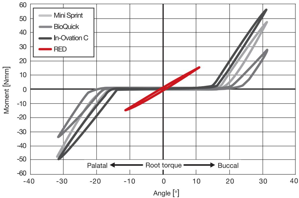
**Figure 3.** Typical graphs of the torque measurements with  $0.018'' \times 0.025''$  ss and conventional twin bracket, passive and active SL bracket in comparison with the elastodynamic bracket with V slot and V wire.
