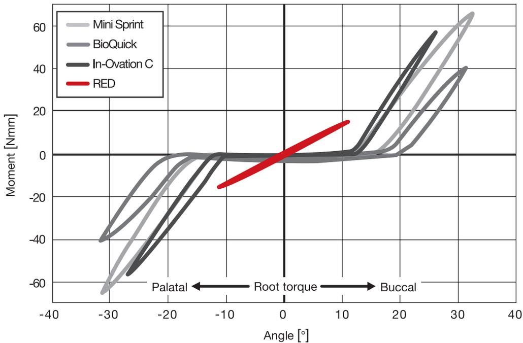
**Figure 4.** Typical graphs of the torque measurements with  $0.019'' \times 0.025''$  ss, conventional twin bracket (Mini Sprint, Forestadent, Pforzheim, Germany), and passive (BioQuick, Forestadent, Pforzheim, Germany) and active self-ligating brackets (In-Ovation C, DENTSPLY Int., York, Pa) in comparison with the elastodynamic bracket with V slot and V wire.
