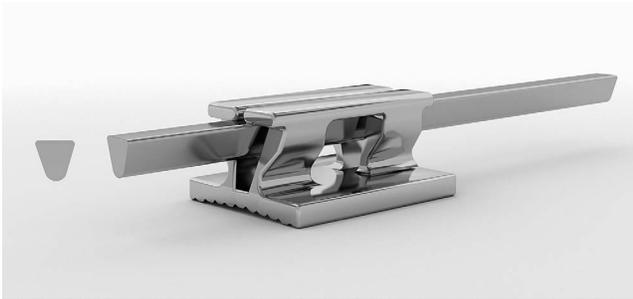
**Figure 1.** Elastodynamic bracket design. Design of the bracket differs from conventional brackets in its slot geometry of a V slot and V wire. This achieves an accurate fit of the wire in the slot. As a result of the V slot, slot-filling archwires can be used for the first time. The monolithic design of the nickel titanium (NiTi) bracket allows for flexible bracket structures and the transmission of small, well-defined moments.
