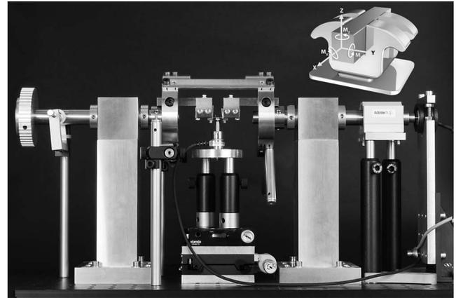
**Figure 2.** Measuring device and coordinate system. The measured data are recorded via the six-axis sensor in all spatial directions and plotted.
