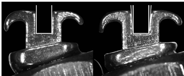
**Figure 6.** Slot deformation after application of torque. There are changes to the slot in the conventional twin brackets and SL brackets, particularly after using the 0.019'' × 0.025'' ss archwire. In contrast, the elastodynamic bracket does not alter its slot shape.
