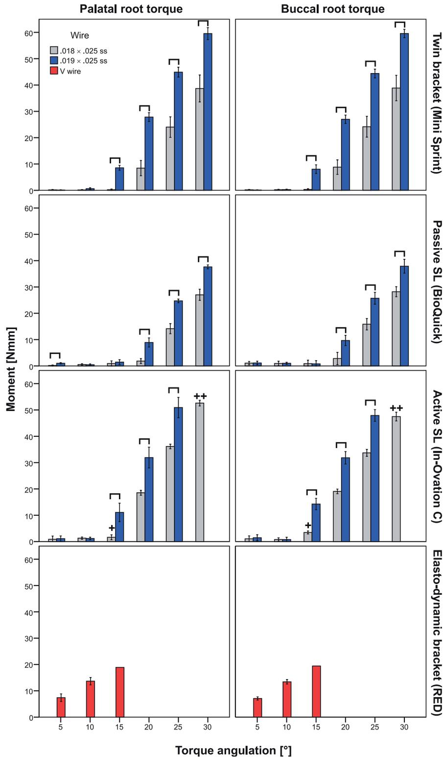
**Figure 5.** Comparison of the moments for palatal and buccal root torque in a conventional twin bracket, passive and active self-ligating (SL) brackets, and 0.018'' × 0.025'' and 0.019'' × 0.025'' ss archwires vs the elastodynamic bracket with V slot and V wire.
