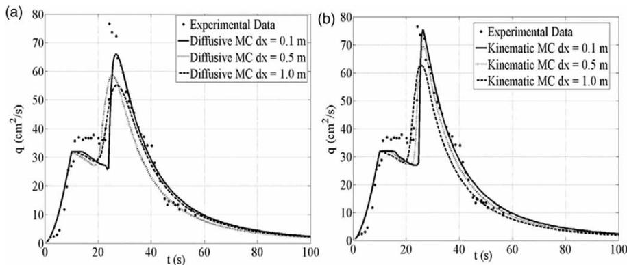
**Figure 6** | Test 3: Flood wave at the channel outlet (rain duration  $t = 10$  s), influence of mesh size on the computed hydrographs using the MacCormack scheme: (a) diffusive, (b) kinematic approximations.
