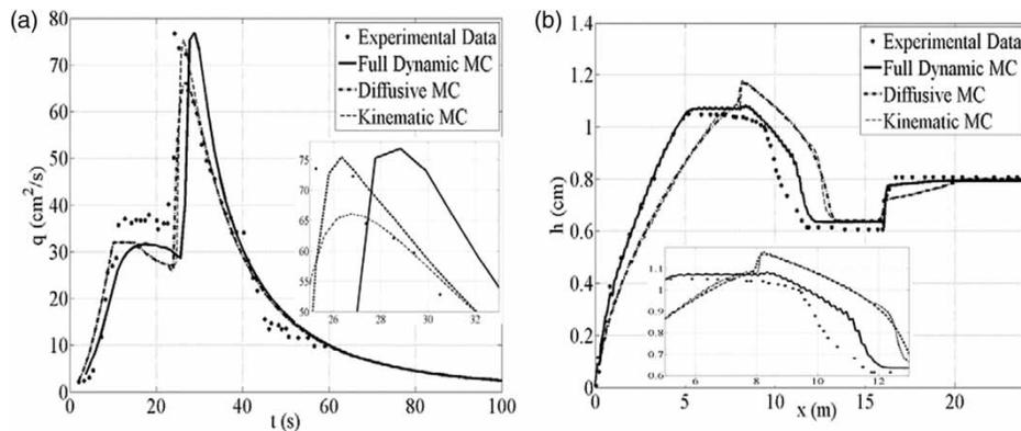
**Figure 4** | Test 3: Comparison of experimental data and numerical results (rain duration  $t = 10$  s): (a) flood wave at the channel outlet, (b) longitudinal water depths profile at the end of the rainfall input.
