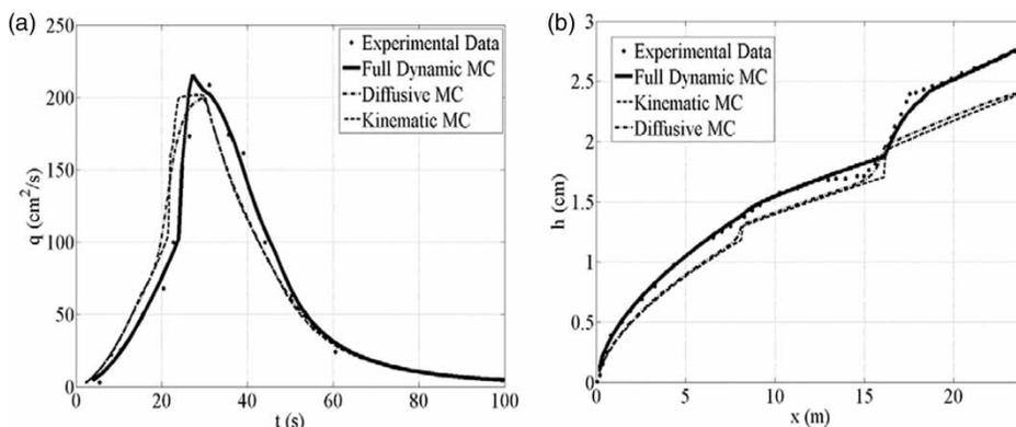
**Figure 3** | Test 3: Comparison of experimental data and numerical results (rain duration  $t = 30$  s): (a) flood wave at the channel outlet, (b) longitudinal water depths profile at the end of the rainfall input.
