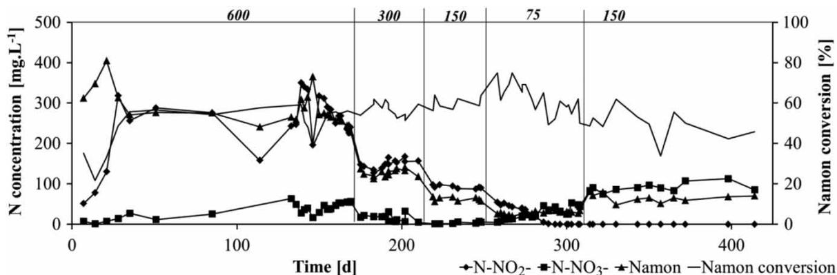
**Figure 1** | Effluent concentrations of TAN,  $\text{N-NO}_3^-$  and  $\text{N-NO}_2^-$  and TAN conversion for SBR I operated at  $15^\circ\text{C}$  and influent concentrations of 600, 300, 150 and  $75 \text{ mg L}^{-1}$  and TAN loading rate of  $0.2 \text{ kg m}^{-3} \text{ d}^{-1}$ .
