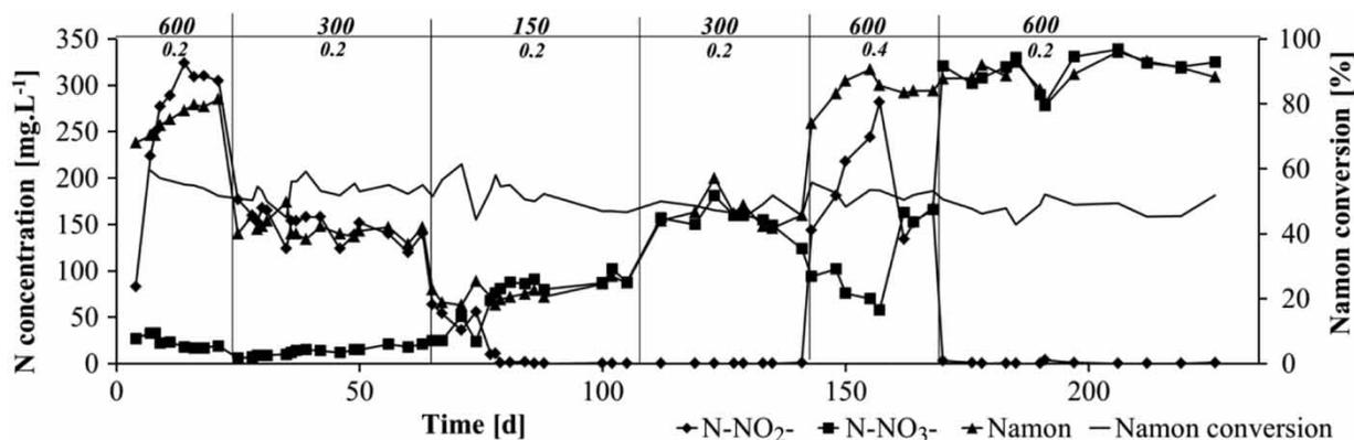
**Figure 2** | Effluent concentrations of TAN,  $\text{N-NO}_3^-$  and  $\text{N-NO}_2^-$  and TAN conversion for SBR II operated at  $21 \pm 1^\circ\text{C}$  and influent concentrations of 600, 300 and  $150\text{ mg L}^{-1}$  and TAN loading rate of 0.2 and  $0.4\text{ kg m}^{-3}\text{ d}^{-1}$ .
