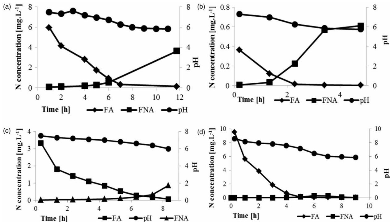
**Figure 3** | The development of FA, FNA and pH during a typical cycle in SBR I (a), (b) and SBR II (c), (d). The influent TAN concentrations were  $600\text{ mg L}^{-1}$  (a),  $150\text{ mg L}^{-1}$  (b),  $300\text{ mg L}^{-1}$  (c) and  $150\text{ mg L}^{-1}$  (d).
