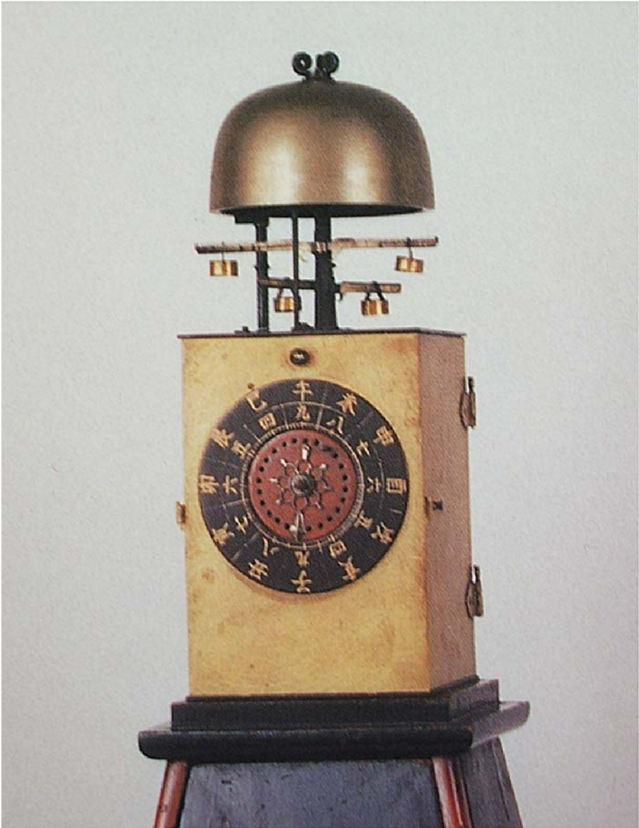
Fig. 1 The type with two foliots ( Nicho Tempu type) [from Sachiko Oda ed., SEIKO Tokei Shiryokan Zo Wadokei Zuroku (Illustrative Catalogue of Japanese Clocks Preserved at the SEIKO Clock Museum) (Tokyo: SEIKO Clock Museum, 1994), p. 25]
