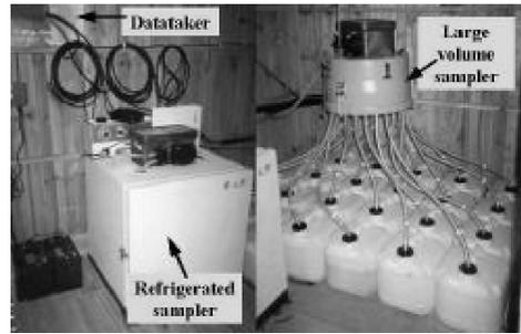
**Figure 4** Sample collection systems, control unit (on wall) and spare bottles
