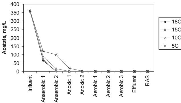
**Figure 3** The uptake of acetate throughout the reactors of the EBPR system
