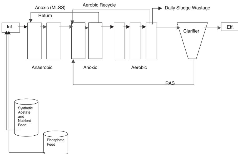
**Figure 1** Flow schematic of the lab-scale UCT system
