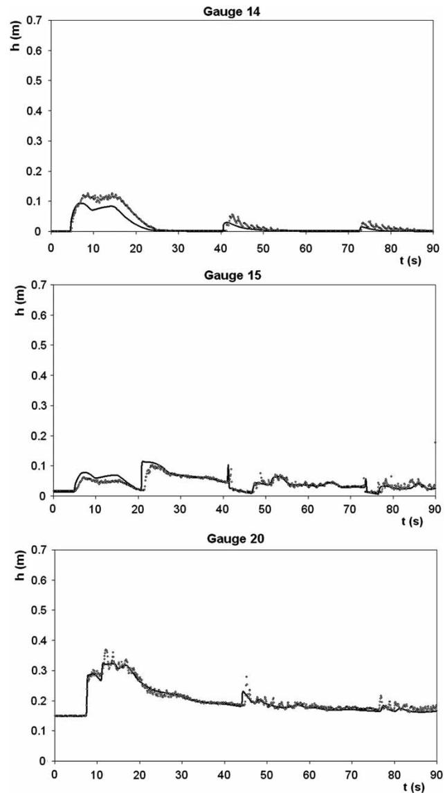
**Figure 4** | Laboratory dam-break experiment: comparison between experimental (circles) and numerical results (continuous line) for gauges G14, G15 and G20 (water depth).
