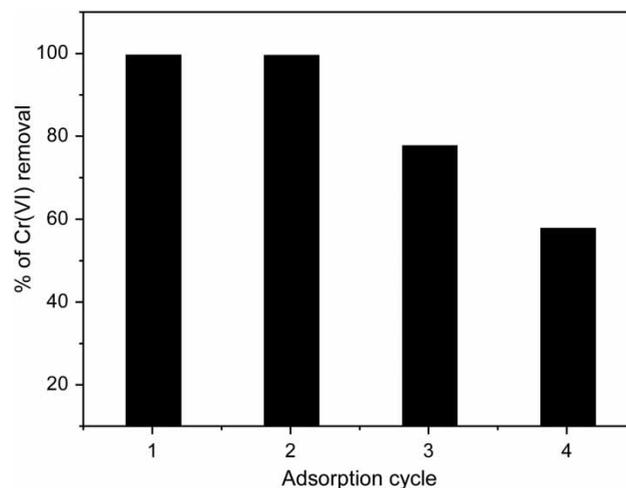
**Figure 5** | Regeneration of PANI/sepiolite for four cycles.
