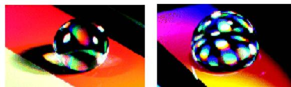
**Fig. 6** Dynamic tuning of surface wetting on a nanostructured hydrophobic surface with application of electrical potential Ref. [30] (a) surface structure produced on a silicon substrate and (b) change in droplet contact angle when an electrical potential is applied
