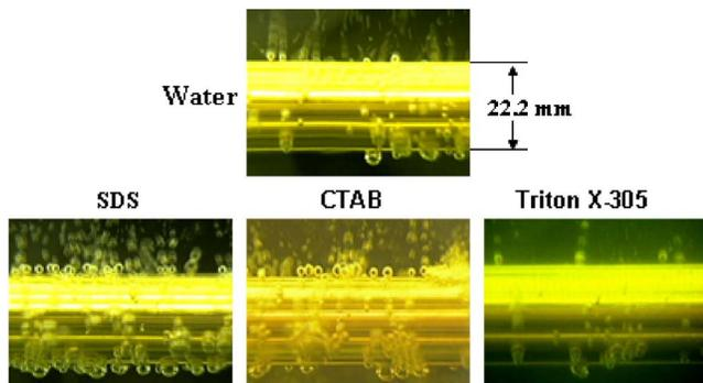
**Fig. 4** Boiling behavior in distilled water, and aqueous surfactant (SDS, CTAB, and Triton X-305) solutions in their respective half-micellar concentrations (or  $C=0.5CMC$ ) and at a heater wall heat flux of  $q''_w=20 \text{ kW/m}^2$
