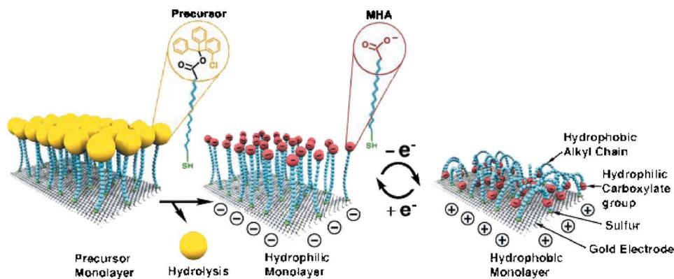
**Fig. 5** Conceptual representation of a “reversibly switching surface” by applying an electrical charge to dynamically tune the orientation of self-assembled molecular monolayers and render the surface hydrophilic or hydrophobic Ref. [62]
